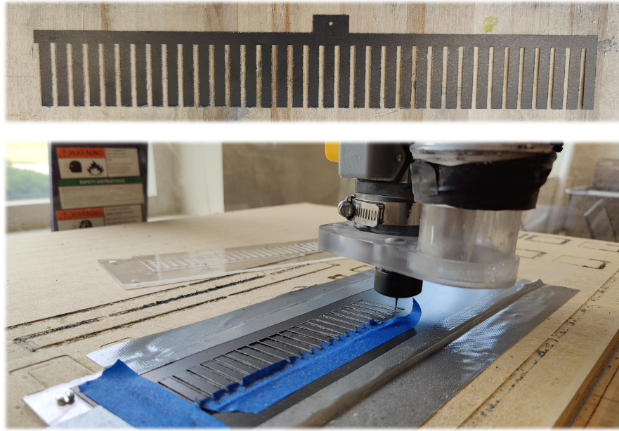
Figure 7.4: Capacitive power transfer strips cut through Shopbot CNC machine
