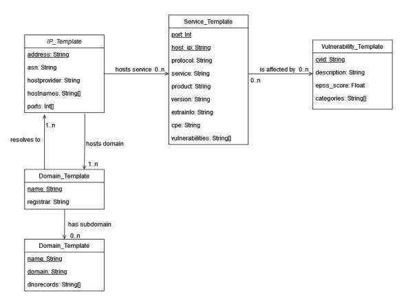
Figure 6.2: Diagram of the data entries initially modeled in the framework.
