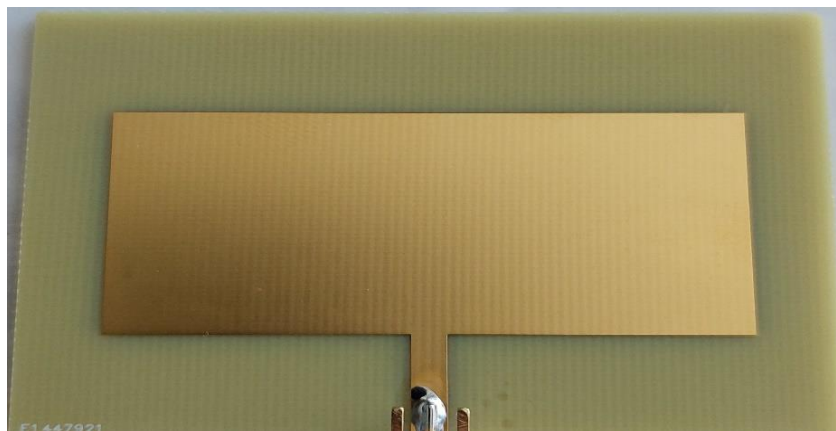
Figure 3.4.4 Photograph of fabricated antenna
