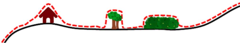
*Figure 18 Continuous black line represents the DTM whilst the DSM is showed as dashed red line [60]*
