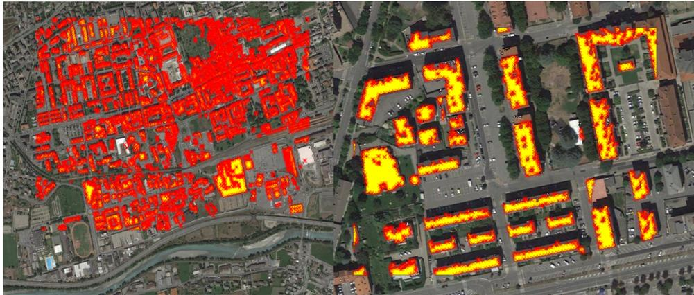
Figure 64 The overall suitable rooftop area calculation by eliminating the areas smaller than 7m<sup>2</sup>
