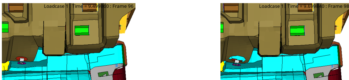
Figure 5.31 – Frame of the threaded connection before (left image) and after (right) the breakage
