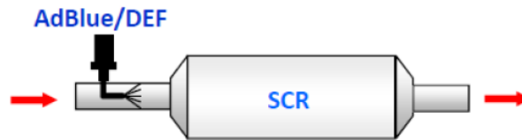
Figure 96 - Aftertreatment system architecture for MD/HD applications [FPT Industrial]
