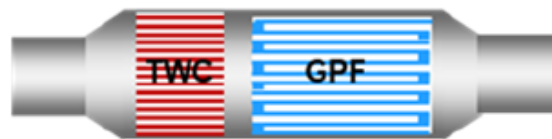
Figure 86 - Euro 6d architecture for passenger cars [29]
