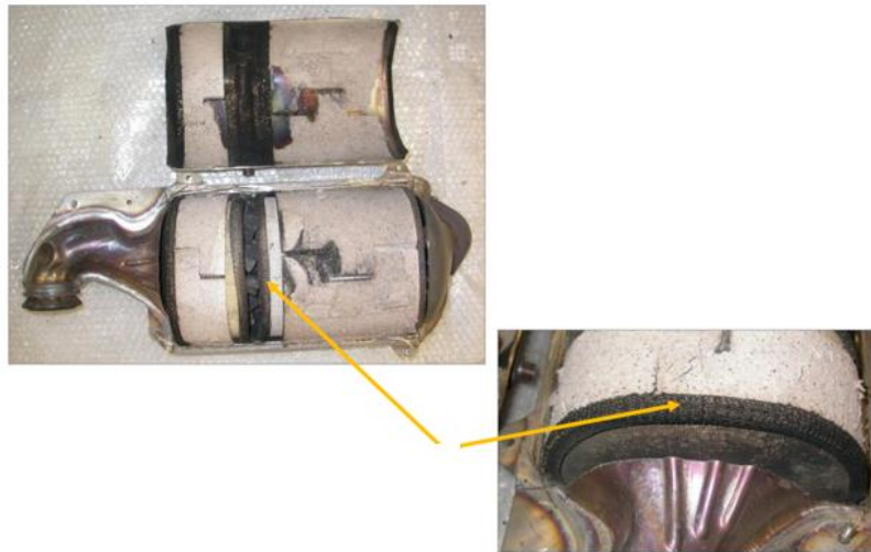
Figure 106 – Visual inspection DPF with wire-mesh elements highlighted
