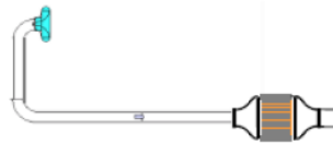
Figure 83 – SI Passenger cars Euro 1/2 after-treatments architecture [FPT Industrial]
