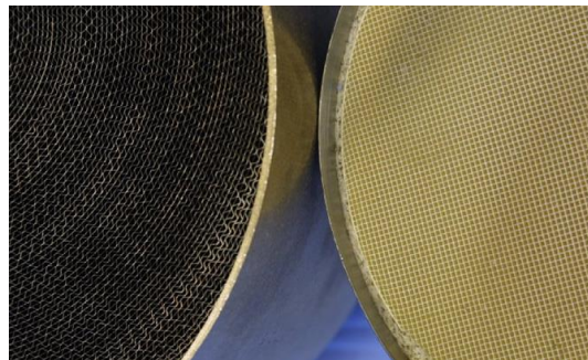
Figure 29 - Examples of a metal foil catalyst substrate and an extruded cordierite substrate [8]
