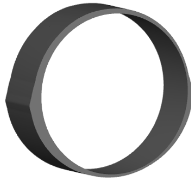
Fig. 5.24 Main bearing lemon shape
