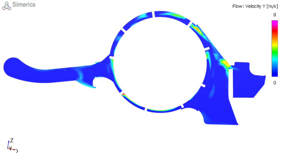
Fig. 6.5 Instantaneous velocity V_y contour of VDVP at 5000rpm and 100°C in steady state
