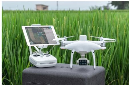
Figura 1.6: DJI P4 Multispectral
