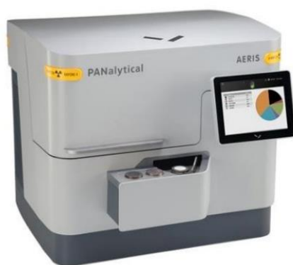
Figura 3.11: Diffratometro XRD – X – Pert Philips PANalytical, Almelo, The Netherlands [112]
