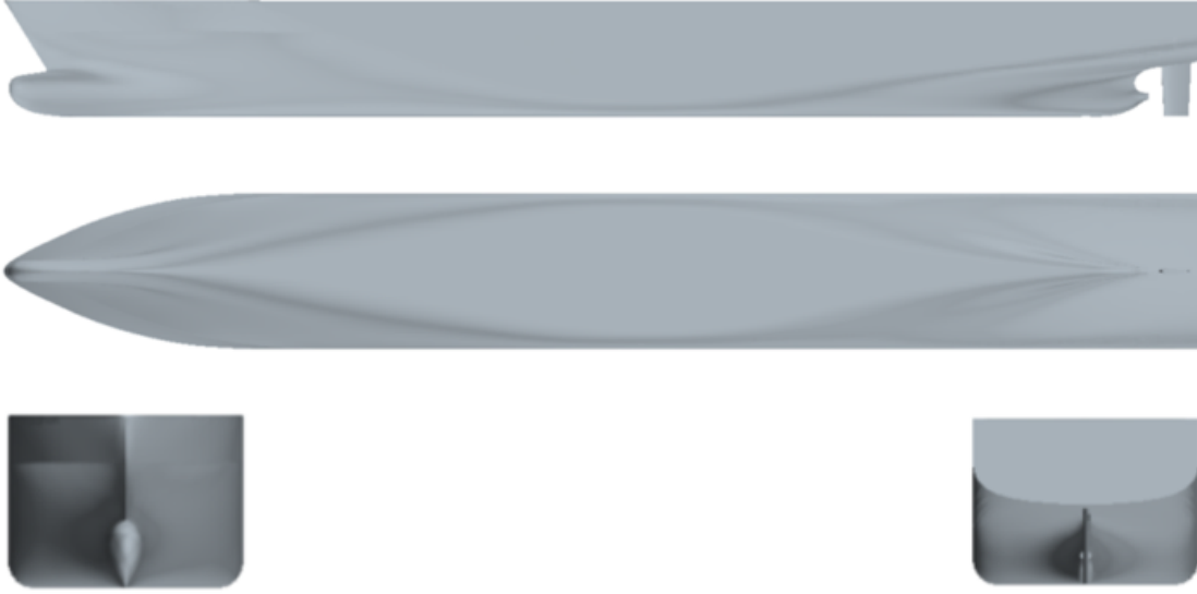
Figure 58: KCS CFD geometry
