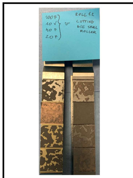
Figure 4.29 Specimens after testing at different testing speeds keeping the other parameters constant (setup 2)
