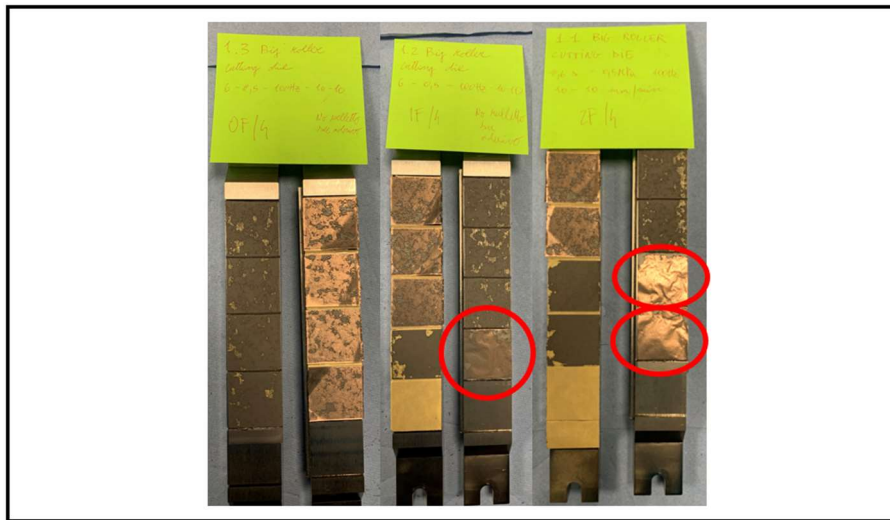
Figure 4.17 Specimens tested with method 1, the three failures are circled in red
