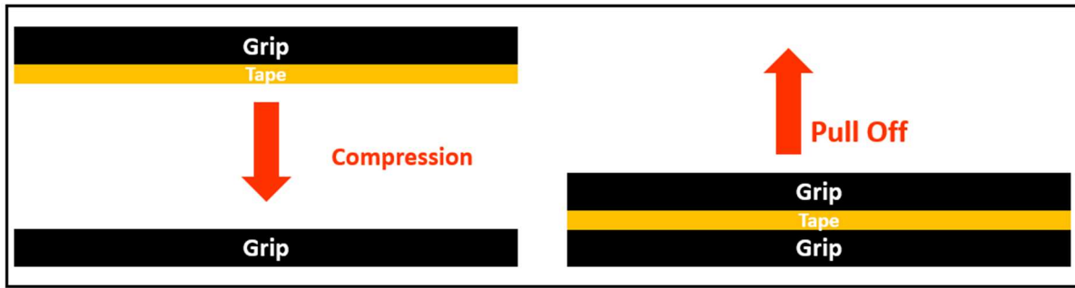
Figure 4.36 Representation of the z-direction pull test to record the adhesion between the tape and the grip
