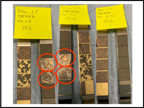
Figure 4.21 Specimens tested with method 1, the four failures are circled in red
