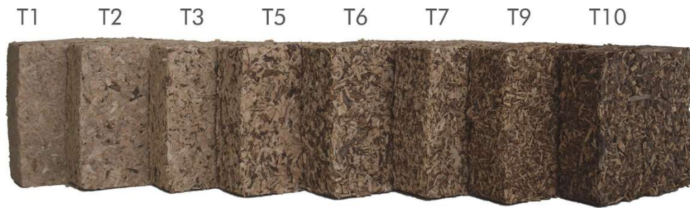
Figure 2. Samples produced with increasing percentage composition of olive wood chips
