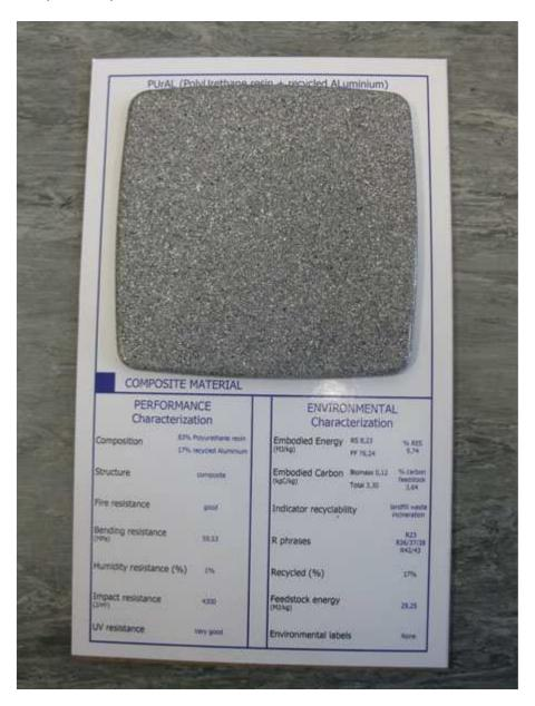
In conclusion, the final results have been very satisfactory and fulfil the expected targets: bending tests and impact resistance tests have provided very interesting data, beyond all the expectations; the moisture testing has proved that the samples do not tend to absorb water in their mass and the UV test has proved that the samples are not sensitive to the ultraviolet radiations.
