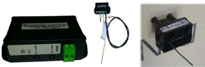
Figura 53. Tipologie dei sensori utilizzati prodotti dalla Omnisense LL (fonte: S. Kordziel, Study of moisture conditions in a multi-story mass timber building through the use of sensors and wufi hygrothermal modeling, tesi magistrale, Colorado School of Mines, 2018, relatore: Dr. Shiling Pei.)
