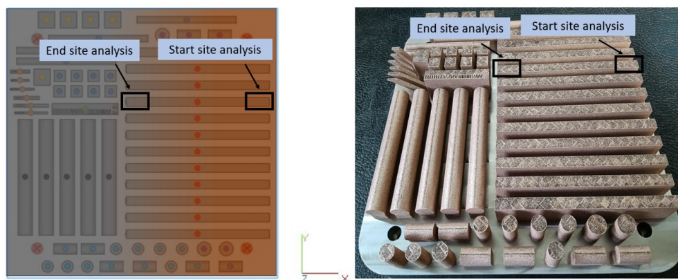
Fig. 8.32 Chemical composition gradient analysis - specimen location on the printing platform
