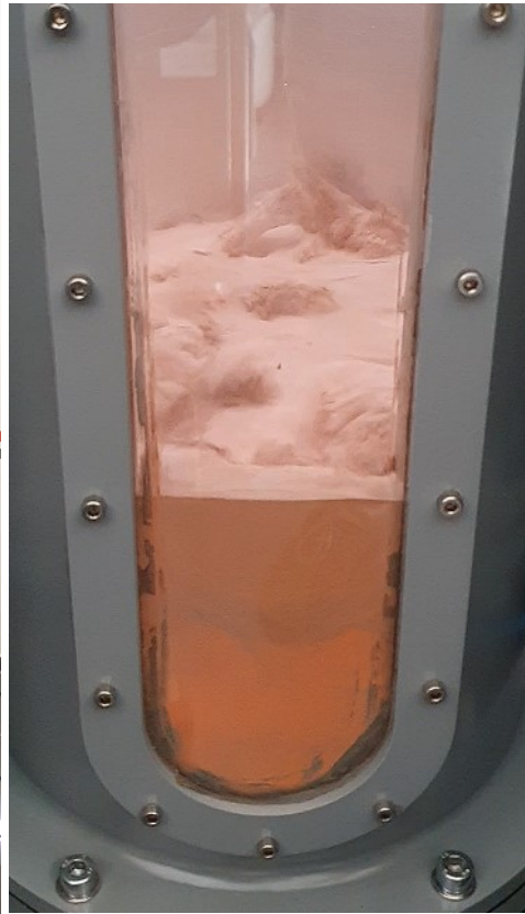
(b) Instant photo of the 'random-boiling' mixing process of the custom Cu17-4PH powder
