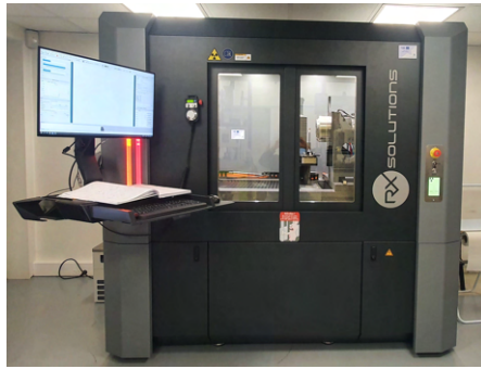
(a) RX Solution EasyTom machine, CERMEL Laboratory of Université de Tours, France (b) Placement of the specimen for the CT scan
