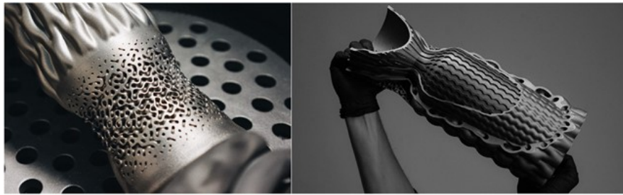
Fig. 2.17 Hyperganic prototype rocket nozzle featuring internal cooling channels and an external lattice, from [8]
