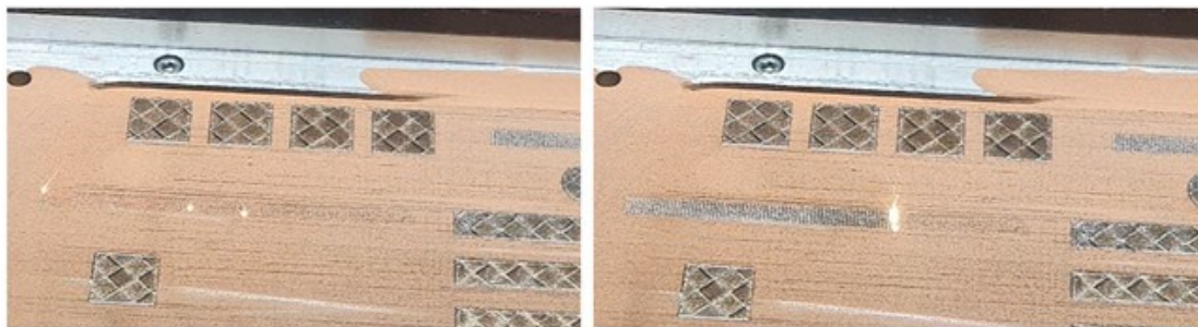
Fig. 5.12 Step A) (left) pre-melting and Step B) (right) Melting process
