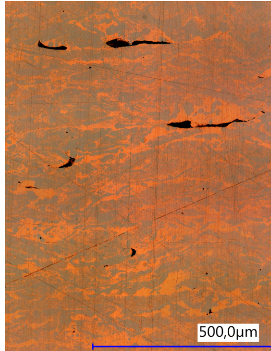
Fig. 8.18 Lack of fusion porosity example
