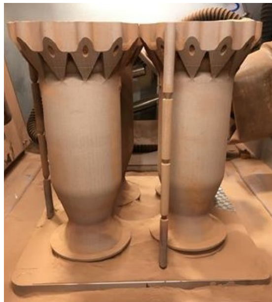
Fig. 2.3 Example of large-scale NASA GRCop-42 chambers fabricated by SLM
