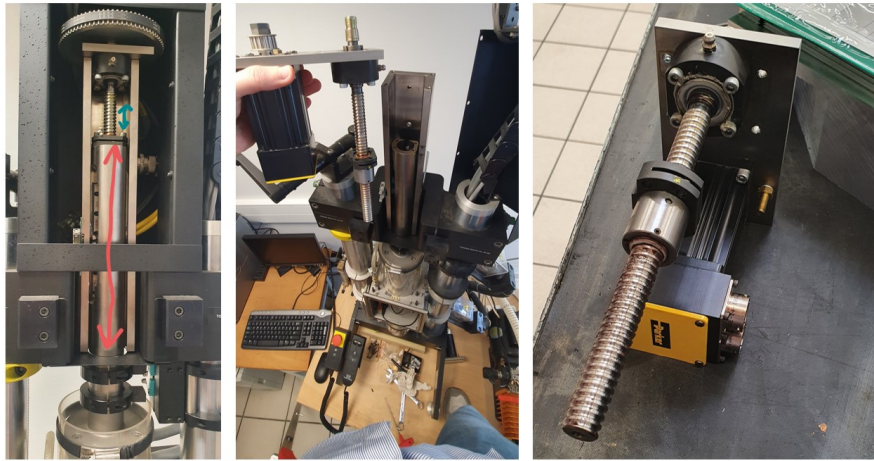
Fig. 6.41 INSTRON ETMT II disassembly procedure
