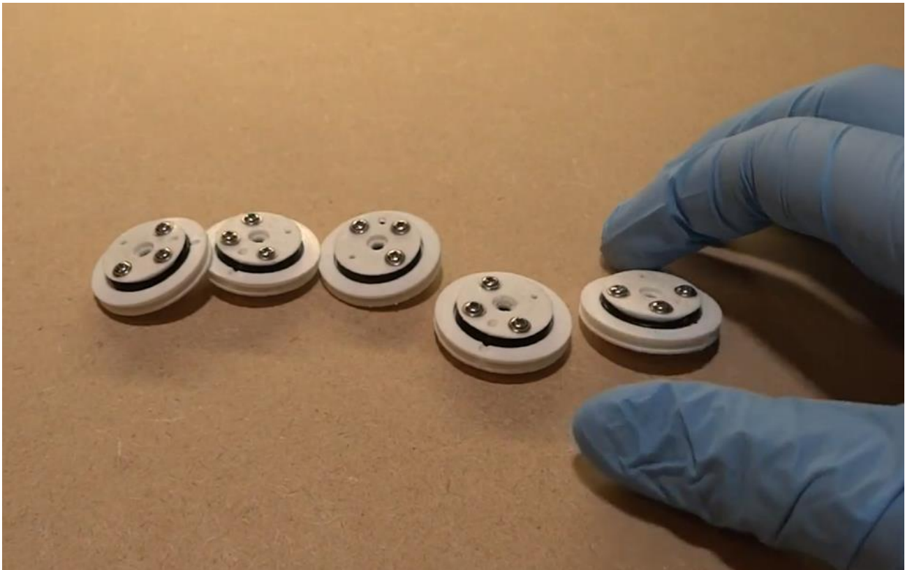
Figure 27: Robring and servo pulleys
