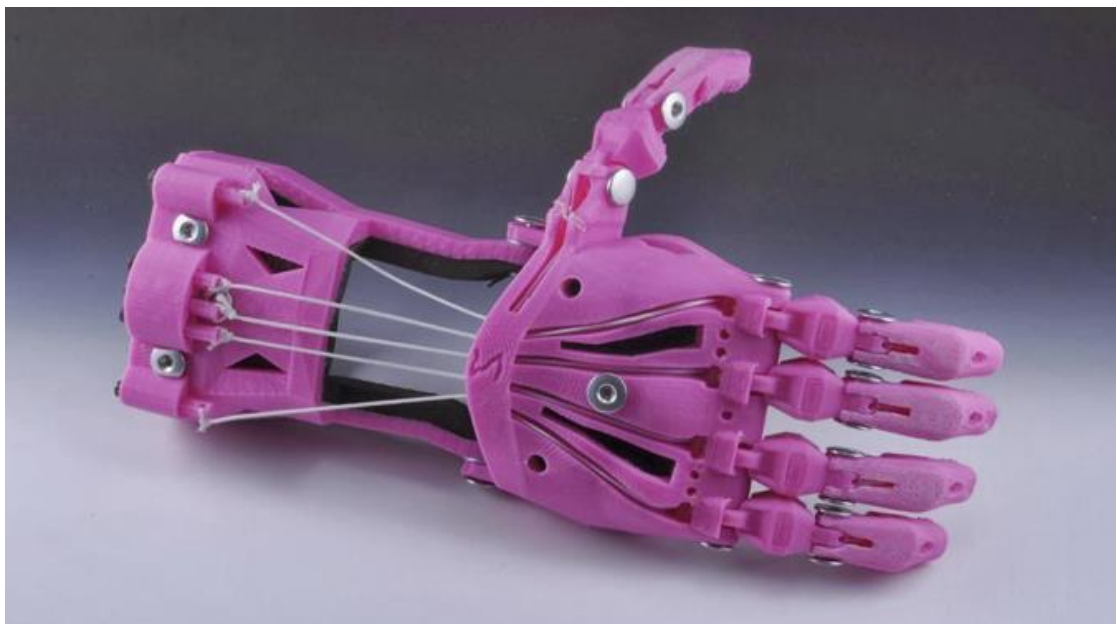
Figure 3: Mechanical powered prostheses with strings
