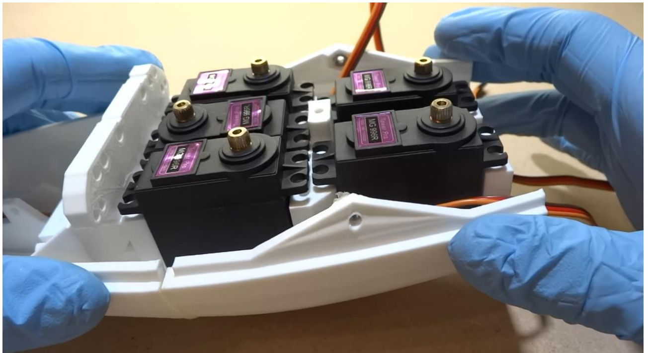
Figure 26: Mounting of the servo
