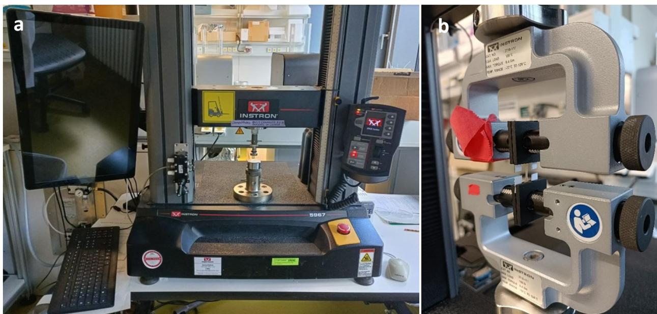
Figure 17. (a) Uniaxial mechanical testing device (Instron 5967, Instron® GmbH, Germany), (b) the tensile strength analysis on the scaffold.
