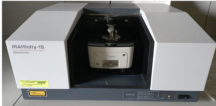
Figure 15. FTIR device (IRAffinity-1S Shimadzu).
