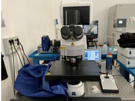
Figura 43: Microscopio a fluorescenza (Zeiss LSM900)
