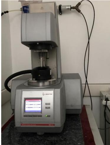
Figure 47: Reometro Anton Paar MCR 102
