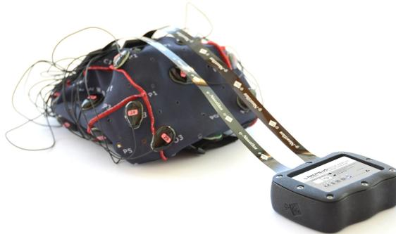
**Figure 2.3:** g.NAUTILUS wearable EEG headset [44].
