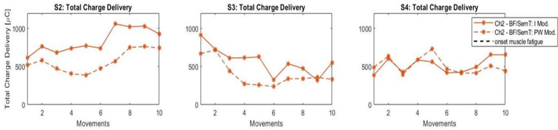
Figure 6.10: Trend of the total charge delivery during the 10 repetitions for each subject and stimulation channel and both types of modulation. Subjects of knee rehabilitation protocol S2, S3 and S4. The dotted black line represents the movement in which muscle fatigue arises.
