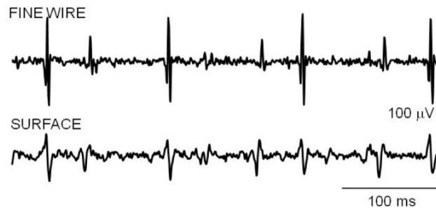
Figure 1.11: Example of intramuscular and surface EMG signals recording. sEMG signal is smoothed and reduced in amplitude by the filtering effect of the subcutaneous tissues [13].
