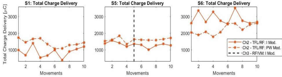
Figure 6.18: Trend of the total charge delivery during the 10 repetitions for each subject and stimulation channel and both types of modulation. Subjects of hip rehabilitation protocol S1, S5 and S6. The dotted black line represents the movement in which muscle fatigue arises.
