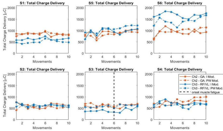
Figure 6.50: Trend of the total charge delivery during the 10 repetitions for each subject and stimulation channel and both types of modulation. Top row: subjects of hip rehabilitation protocol (S1, S5, S6). Bottom row: subjects of knee rehabilitation protocol (S2, S3, S4). The dotted black line represents the movement in which muscle fatigue arises.
