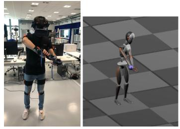
(a) Virtual simulation of a(b) postural prediction of the user screwing screwing task
