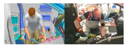
Figure 3.9: Example of how mocap technologies can be used in manufacturing field: the user wears Xsens technology for motion capture while is performing work actions. The movement is digitally reconstructs and then an ergonomic assessment is performed using JackSiemens. Source: [69]
