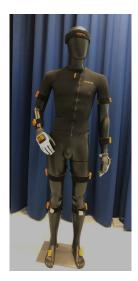
Figure 3.8: XSens an example of inertial system for motion capture
