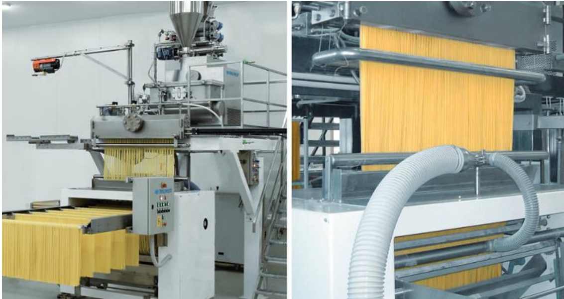
Image 6: Automatic machine for shaping long pasta (Source: https://www.italpast.it/ ).
