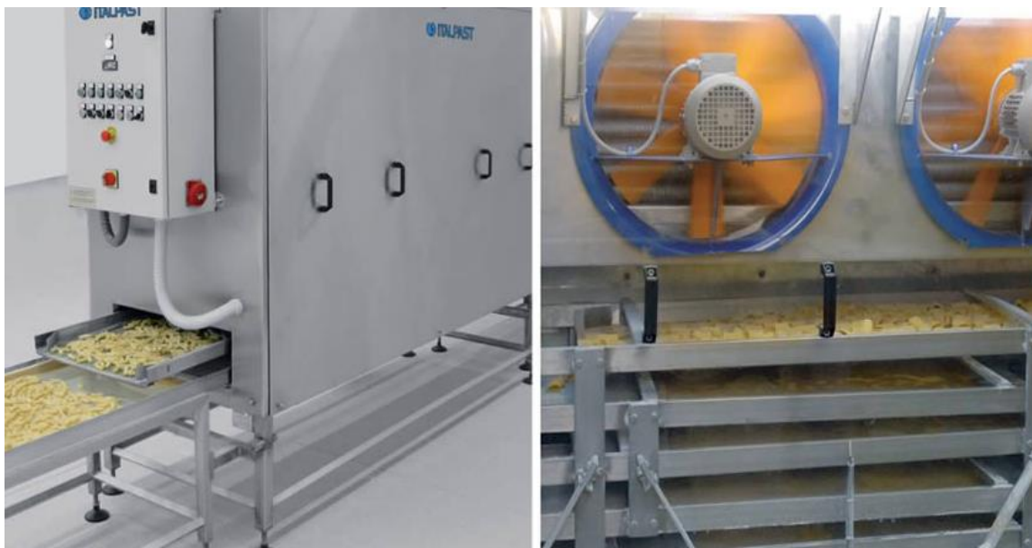
Image 7: heating machine used during the drying phase pasta (Source: https://www.italpast.it/ ).
