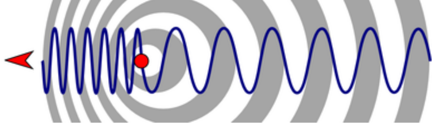
Figure 4.2: Radio wave signal which changes frequency due to Doppler effect caused by the movements of the detect objects [97]
