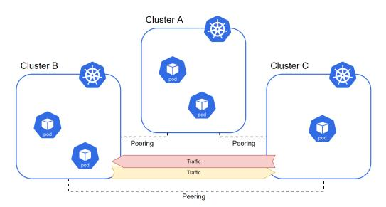
Figure 4.4: Establishing another full peering between the two leaf clusters; traffic can be routed directly to the destination.
