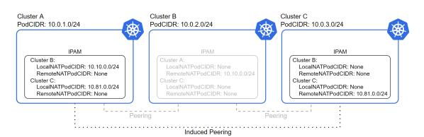
Figure 5.7: IPAM status once the networking setup has completed
