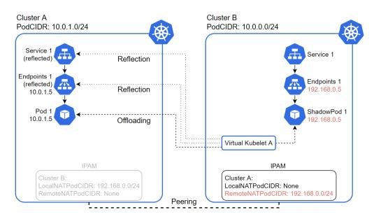
Figure 4.7: Advanced reflection in a two-cluster deployment
