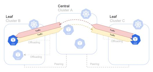
Figure 4.3: Traffic is routed through the central cluster
