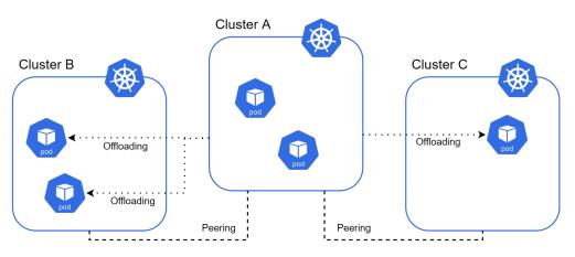
Figure 4.2: Three-cluster deployment
