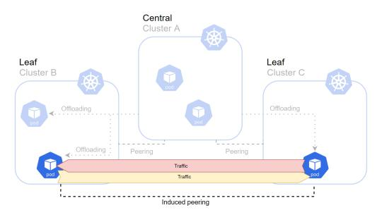
Figure 4.5: Induced peering between the two leaf clusters; traffic is routed directly to the destination.
