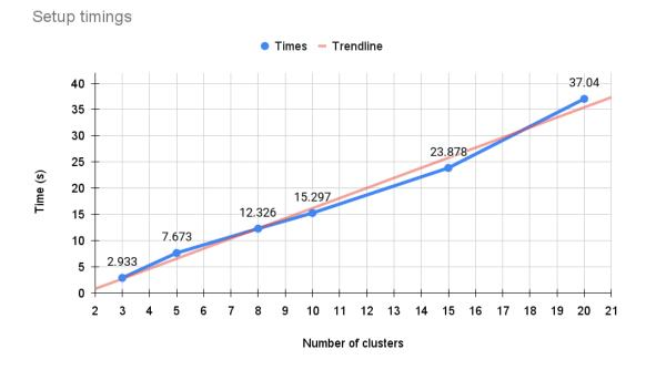
Figure 7.5: Time to setup a full mesh of induced peerings
