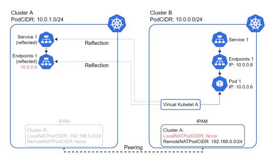
Figure 4.8: Alternative reflection in a two-cluster deployment
