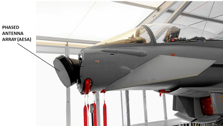
Figure 1.6. The Eurofighter Typhoon combat aircraft with its nose fairing removed, revealing its Euroradar CAPTOR AESA radar antenna. Active Electronically Scanned Array (AESA) is a computer-controlled phased antenna array, which means that the beam of radio waves can be steered to different directions. (source: Wikipedia)
