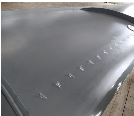
Figure 5.2: Vortex generators on BS Prime wing
