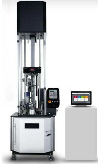
Figure 1.8: An example of Drop Tower
