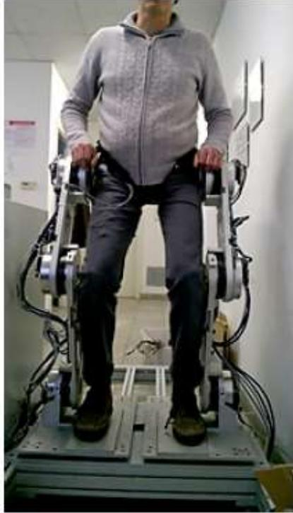
Figure 4-1: Frontal view of the prototype exoskeleton coupled with human user. Reprinted from [24]
