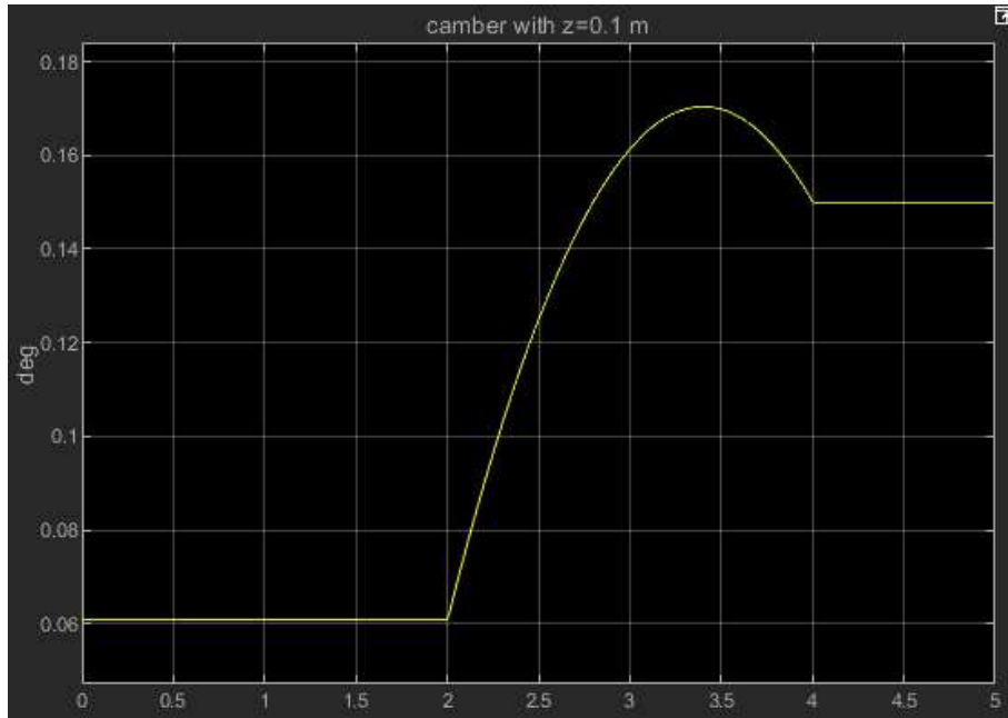
Figure 4.6. Camber angle variation in relation to 0.1 m of vertical displacement
