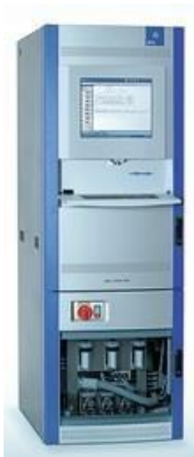
Figure 26: AVL AMA i60 emission bench
