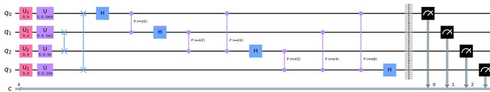
(c) Quantum Fourier Transform circuit (4 qubits) used in the injection
