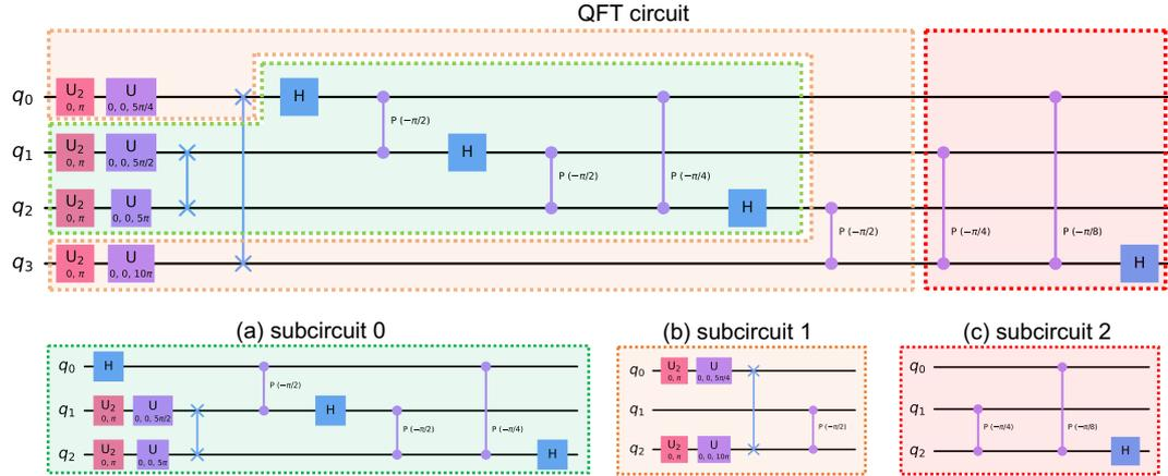
**Figure 5.1:** Original 4-qubit QFT circuit (top) and the three subcircuits of 3 qubits each (bottom) obtained from circuit cutting. The three cuts output combination provides the original circuit output, allowing the cuts to be executed on quantum computers with fewer qubits. Source: [15]
