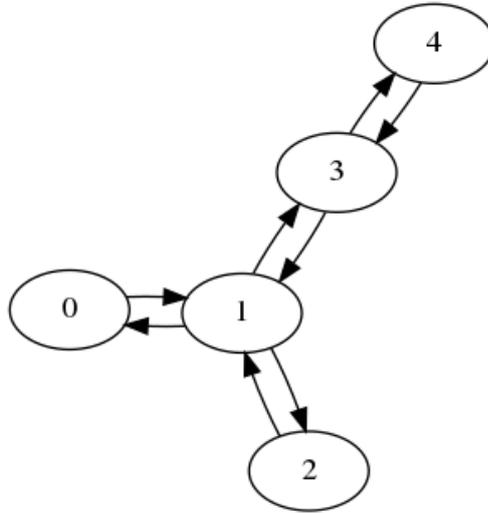
**Figure 6.2:** IBM’s Vigo *coupling map*, indicating its topology. In this work this is used to select where the second fault propagates.
