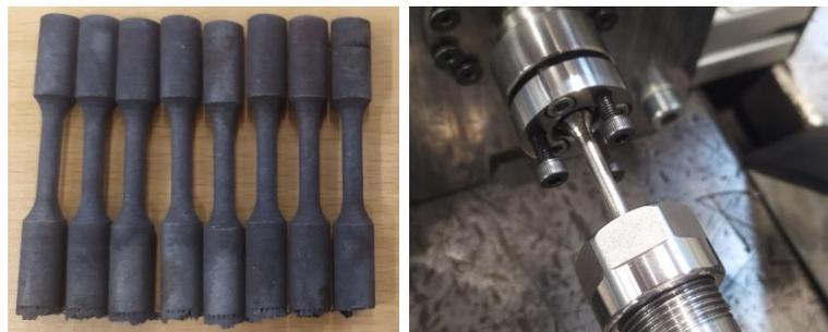
Figure 3. 10: As built specimens and a surface grinded specimen mounted on the machine
