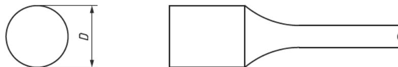
Figure 3. 6: Circular specimen end
