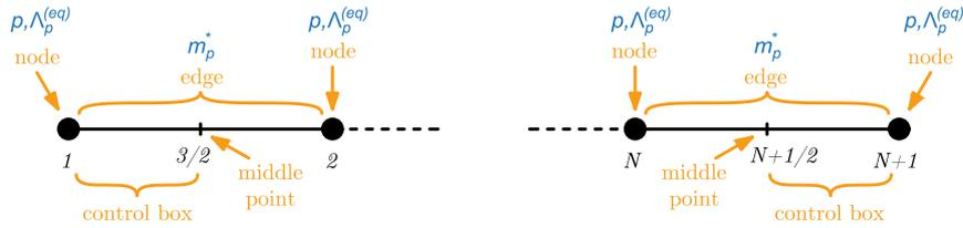
Figure 10.10: Discretization of the boundary conditions to the hole density gradient equation
