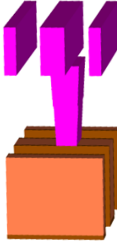
Figure 1.11: 3D structure from SPX showing top via misalignment
