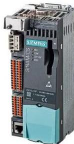
Figure 2.5. CU310-2 PN control unit
