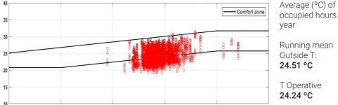
Fig 4.147 Operative Temperature Vs Running Mean Temperature during occupied hours
