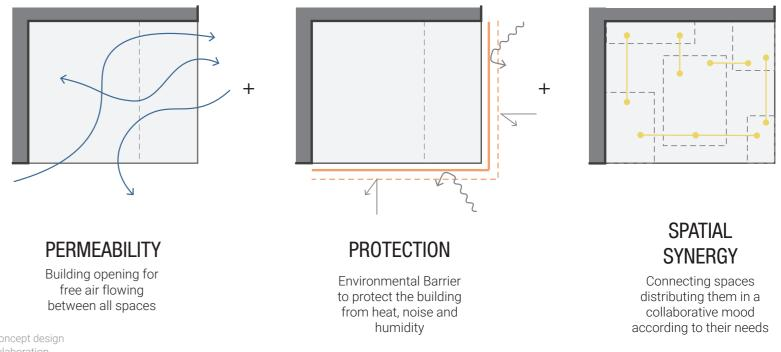
**Fig.6.3** Diagram concept design **Source:** Author's elaboration
