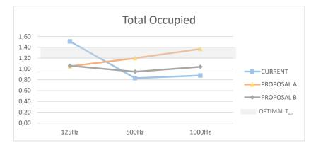
Fig 7.67:Comparison total Occupied room Reverberation time between current and proposals. Source: Author's elaboration
