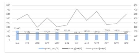
Fig 7.29:Comparison Airflow Current state vs requirements Source: Author's elaboration
