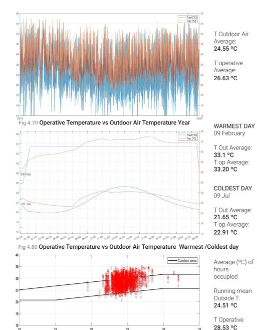
Fig 4.82 Operative Temperature Vs Running Mean Temperature during occupied hours
