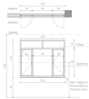
Fig 4.28 Window W1plan and facade \_Scale 1:50/Source: Author's elaboration
