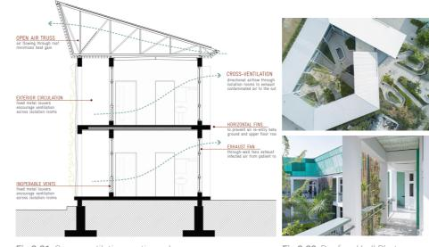
Fig 3.21: Cross ventilation section scheme Source: https://massdesigngroup.org
