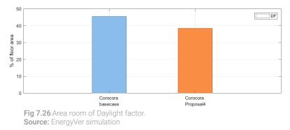
on the east façade was reduced to reduce the glare and the amount of solar radiation. Although a new window has been located in the south-east façade, the results show a daylighting decrease.
