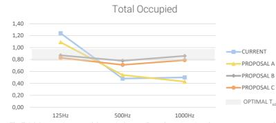
Fig 7.34:Comparison total Occupied room Reverberation time between current and proposals. Source: Author's elaboration
