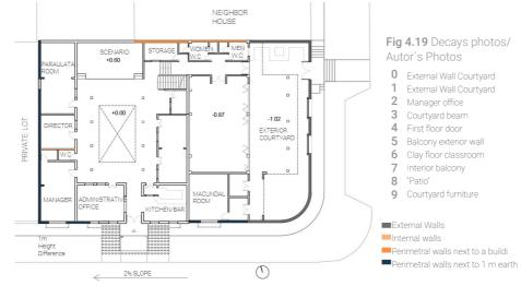
Fig 4.20 Type of walls scheme plan/ Author's elaboration
