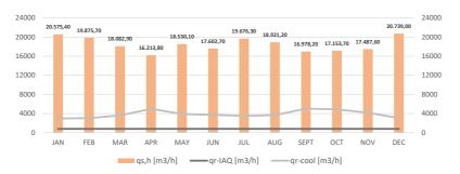
Fig 7.63:Comparison Airflow proposal vs requirements Source: Author's elaboration
