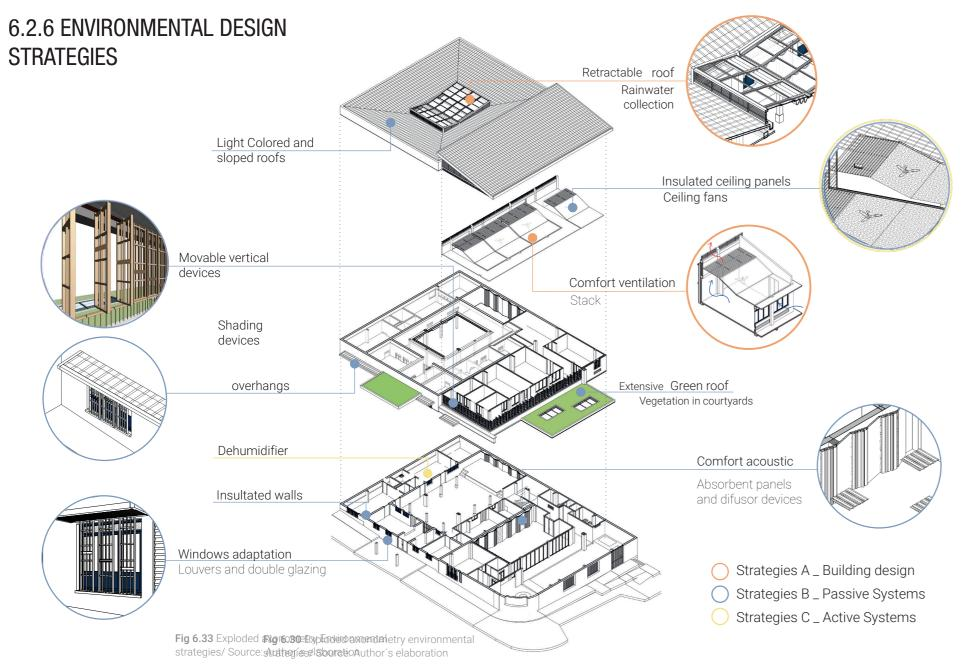
Based on the matrix of problems and solutions, and taking into account the design criteria for hot-humid climate discussed in the chapter 3, the proposal has been designed with strategies from 3 different approaches: Building design, Passive systems and Active systems.
