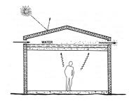
Fig 3.12 Indirect evaporative Cooling Source: Lechner 2008, p.288
