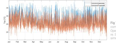
Fig 7.21:Thermal comparison char. Operative temperature. Source: EnergyVer simulation
