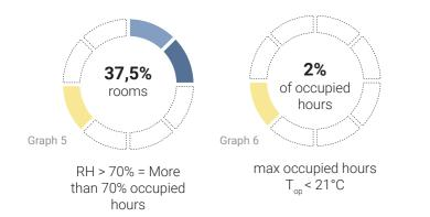
Graph 5: : Taking into account 70% as an acceptable limit of relative humidity the results have shown 37.5% of the rooms are over this limit average in more than 70% of the occupied hours in the year. The rooms with lower indoor temperatures presented high levels of relative humidity: Manager office. "Macundal" classroom and "Paraulata" room.
