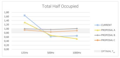
**Fig 7.33**:Comparison Half occupied room Reverberation time between current and proposals. Source: Author's elaboration
