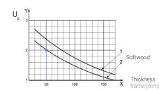
Fig 4.26 Wood frame Ug reference / Source: EN ISO 10077-1, 2017
