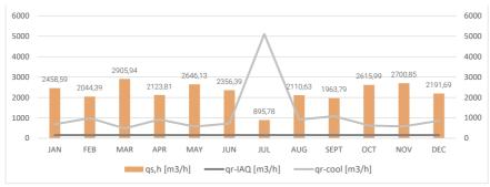
Fig 7.30:Comparison Airflow proposal vs requirements Source: Author's elaboration
