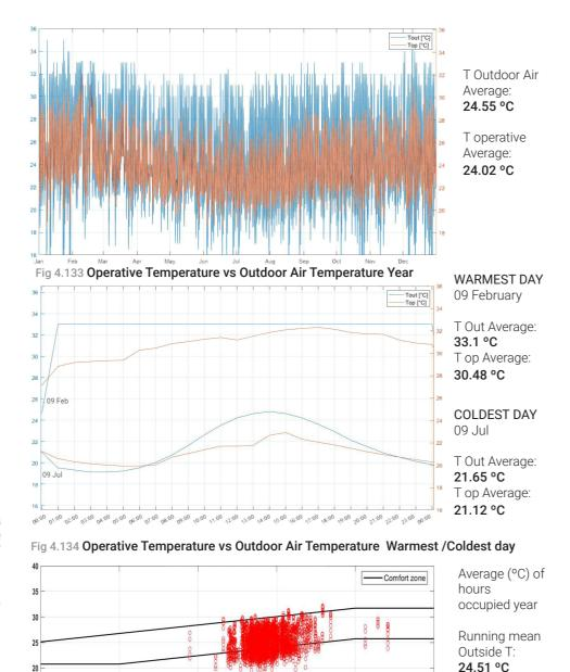
Fig 4.135 Operative Temperature Vs Running Mean Temperature during occupied hours
