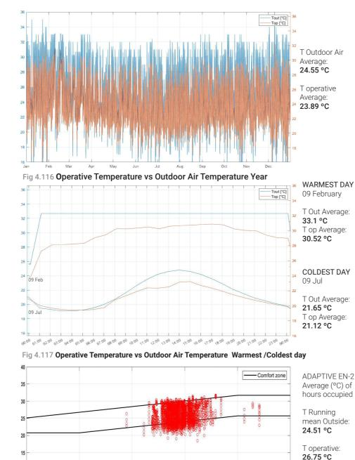
Fig 4.118 Operative Temperature Vs Running Mean Temperature during occupied hours
