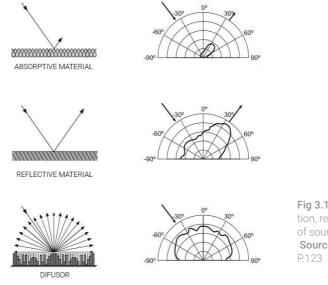
Fig 3.10 Effects of absorption, reflection and diffusion of sound Source: Carrión, A .1998. P.123
