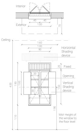
Fig 4.30 Window W2 plan and facade \_Scale 1:50/Source: Author's elaboration
