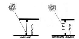
Fig 3.14 Horizontal shading devices Source: Lechner, 2008.p. 400
