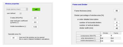
Fig 7.44: Windows properties. Glass and frame Source: EnergyVer simulation
