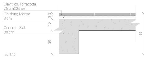
**Fig 4.44** Section Floor/ Source: Author's elaboration
