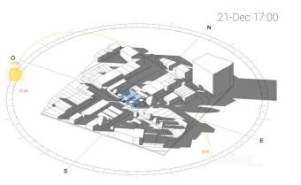
Fig 2.33: Sun Path and shadowing of the context at 17:00 (Winter solstice) Source: Author's elaboration
