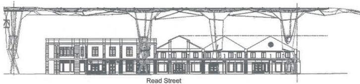
fig. 15 Street section showing canopies projecting above roof height
