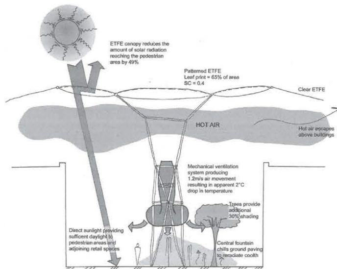
The canopy projects above roof-top height to allow breezes from the river to permeate the urban streets. This breeze is augmented by air blowers that increase the air movement. The structural support of the canopy incorporates fans into the design to provide a low-energy method of increasing air velocity at the street level.
