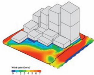
fig. 31 Microclimate simulations' results
