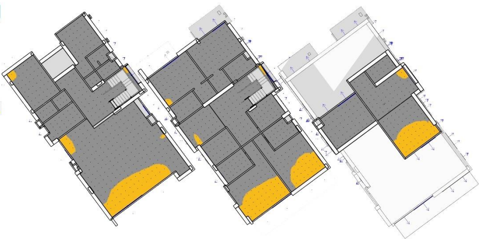
Fig(62): The simulation for UDIa, SDA, ASE and blinds closed percentage in Turin in case study 3
