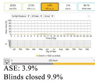
Fig(66): The simulation for UDIA, SDA, ASE and blinds closed percentage in Turin in case study 4
