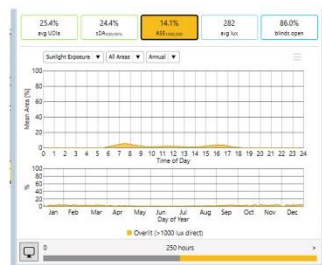
Fig(69): The simulation for UDIA, SDA, ASE and blinds closed percentage in Cairo in case study 5
