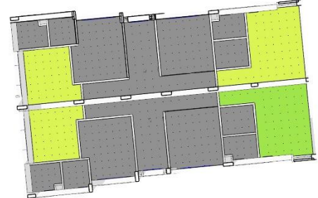
Fig(73): The simulation for average illuminance and daylight factor in Turin in case study 5
