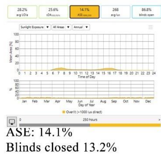
Fig(53): The simulation for UDIA, SDA, ASE and blinds closed percentage in Cairo in case study 1
