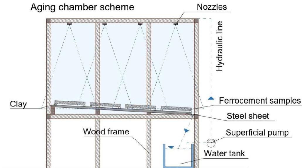
Figure 55 Aging chamber scheme
