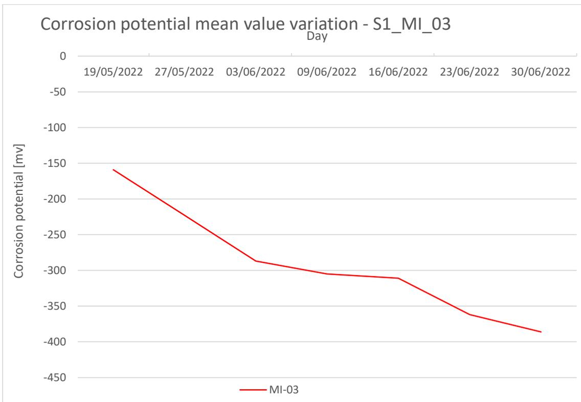
Figure 75 S1-M1-03 corrosion potential mean values
