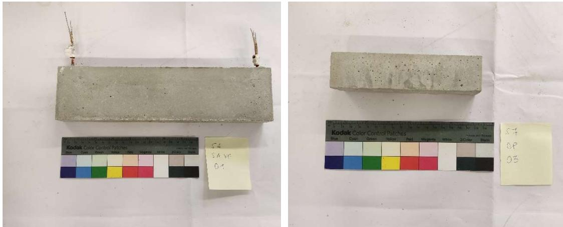
*Figure 41 (on the left) ferrocement sample, (on the right) cement sample*
