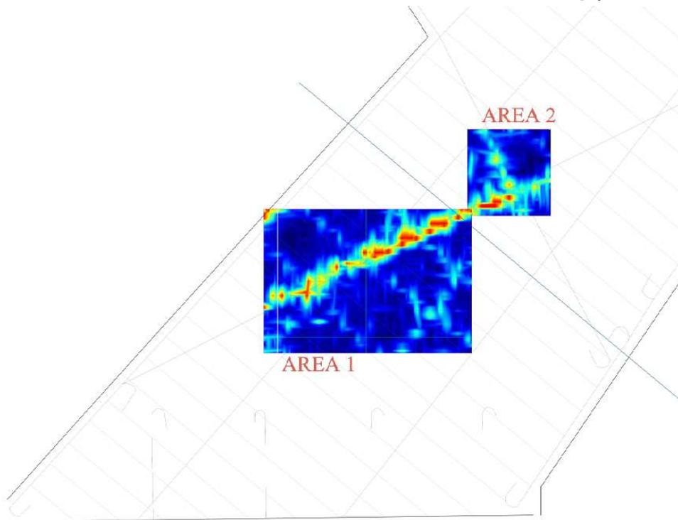
Figure 34 Georadar scan, zoom of the scan PT\_P12N
