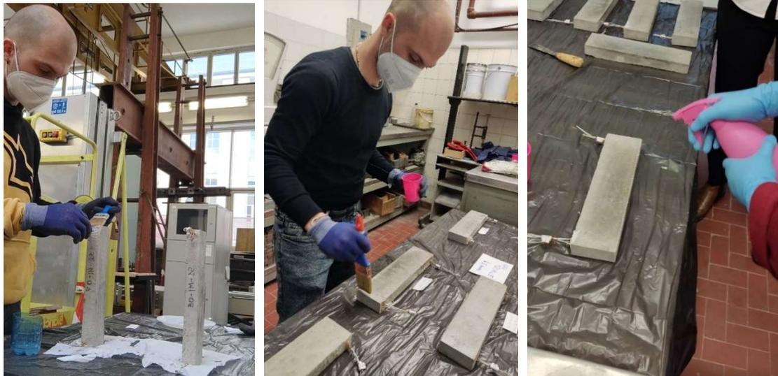
Figure 51 From left: epoxydic resin application, migrant corrosion inhibitor brush application, migrant corrosion inhibitor spray application
