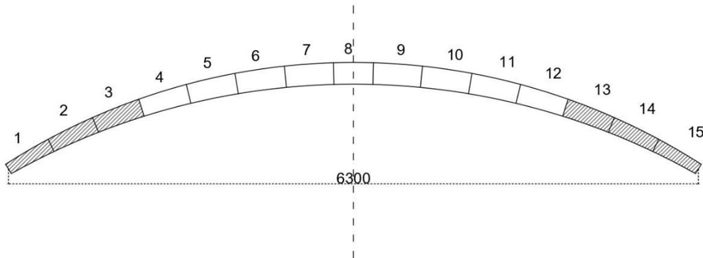
Figure 23 Ferrocement elements scheme
