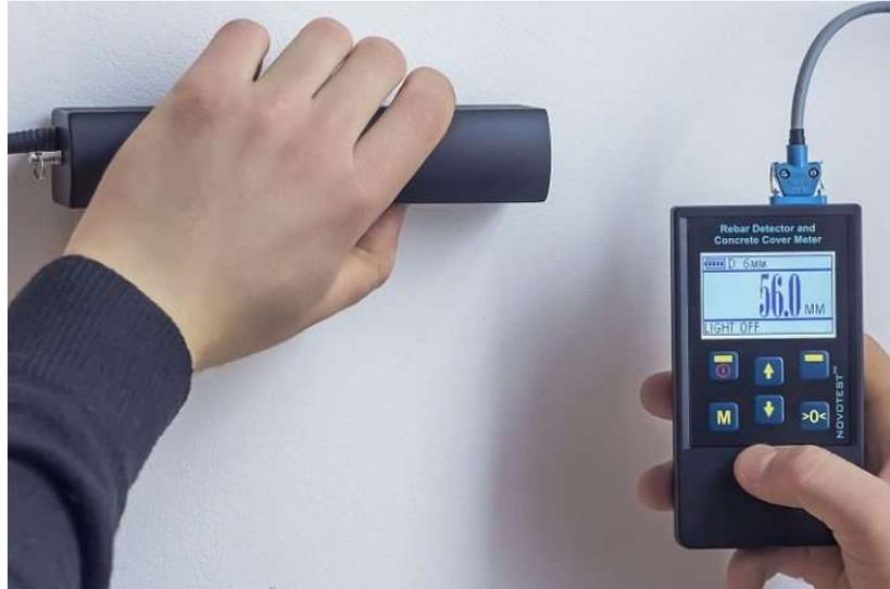
*Figure 11 Cover meter during usage [19]*
