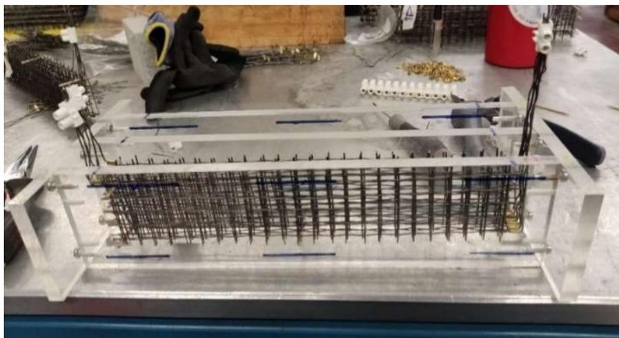
Figure 47 Steel net formwork positioning
