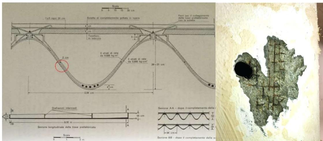
Figure 39 Ferrocement sample position section (on the left), beam after the sample extraction (on the right)
