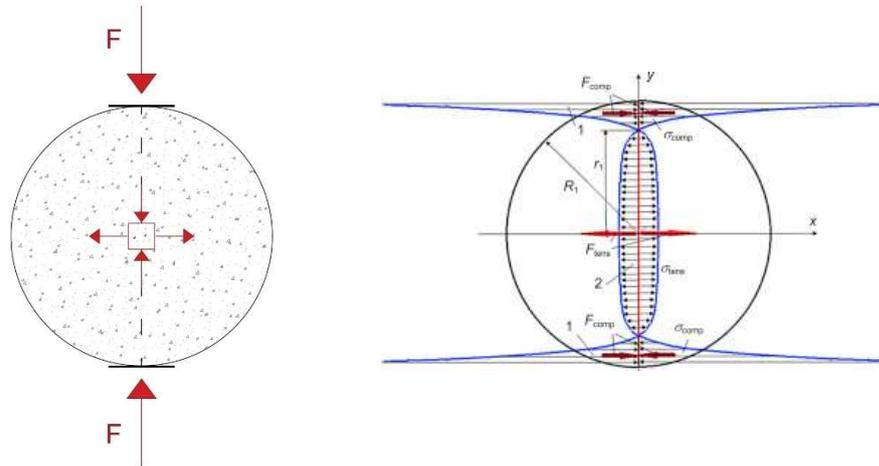
Figure 20 Undirect tension test, forces scheme and [31] stress schemes
