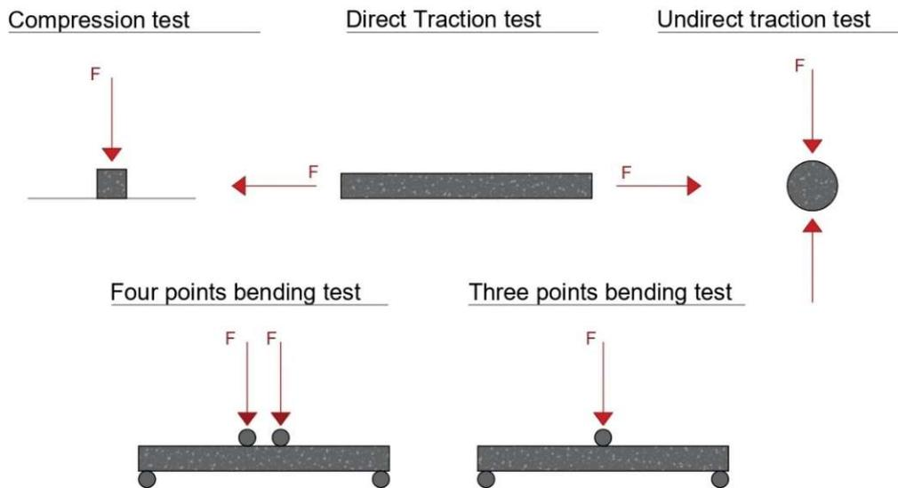
Figure 21 Mechanical tests scheme
