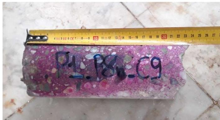
*Figure 16 Feno Naftalin test on concrete sample*
