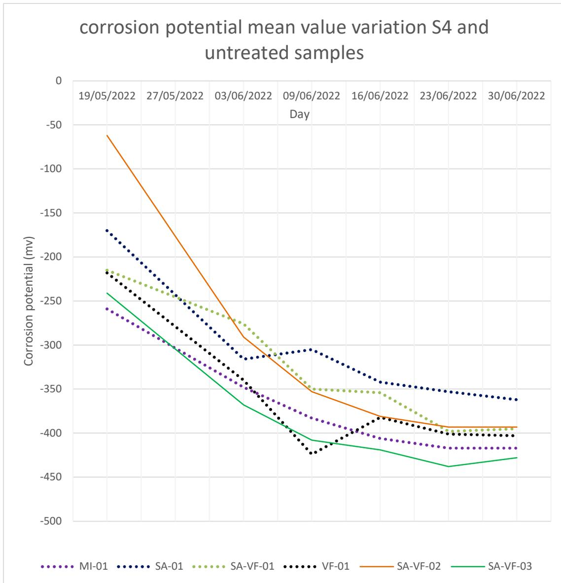
Figure 70 S4 and untreated samples corrosion potential mean values variation
