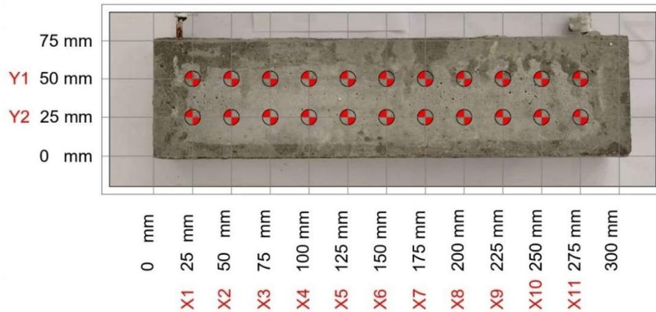
Figure 72 corrosion potential measurements scheme
