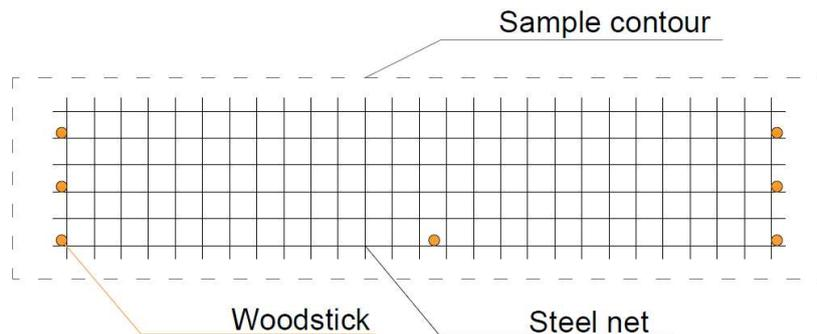
*Figure 44 Steel net and wood sticks positioning*
