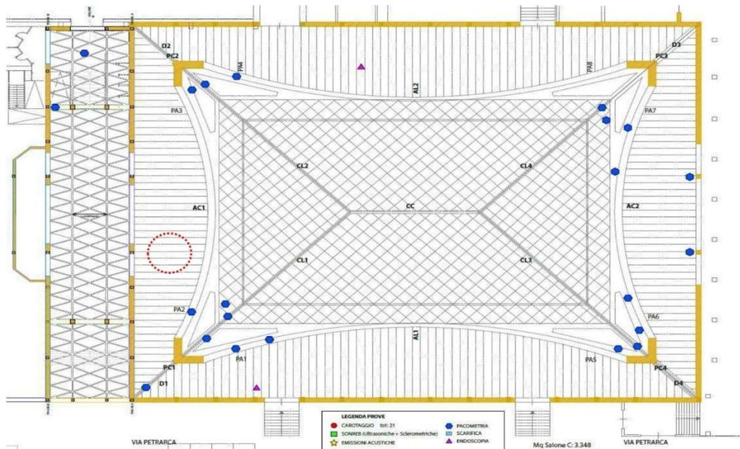
Figure 38 Ferrocement sample position map
