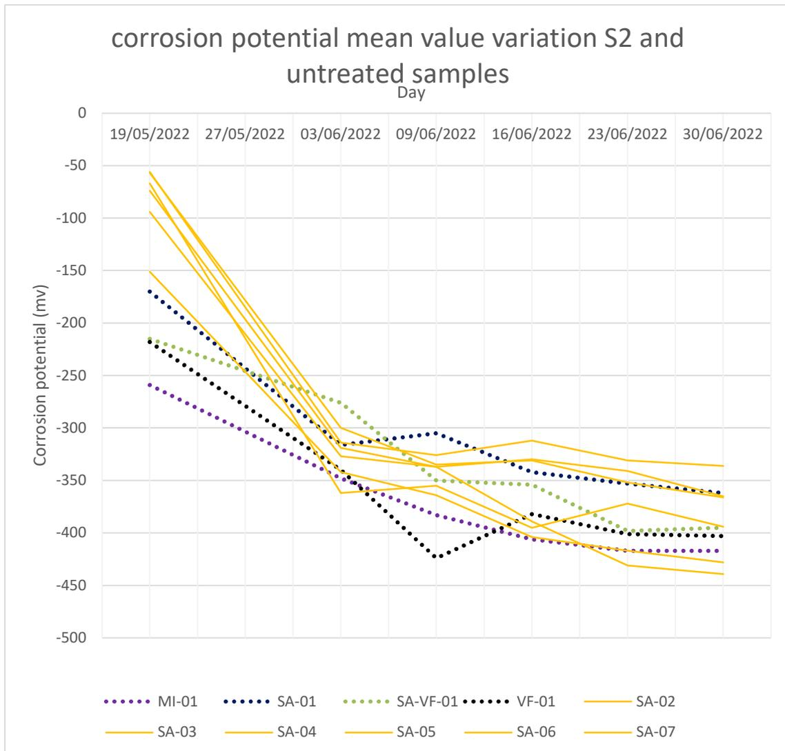
*Figure 67 S2 and not treated samples mean corrosion potential variation*
