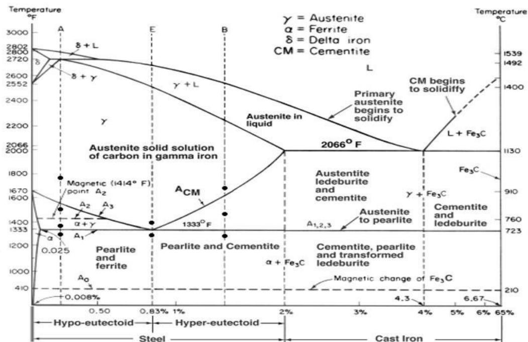
Figure 2 Fe-c phase diagram
