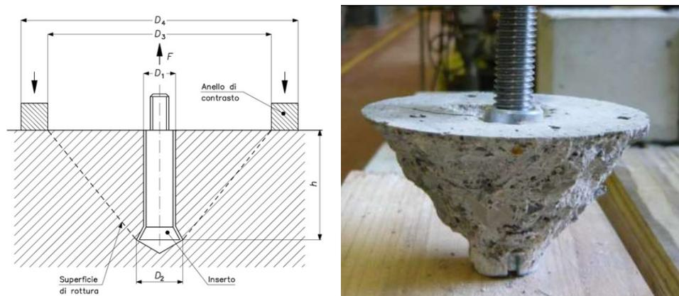
Figure 17 [26] Pull-out test scheme and pull-out cone scheme
