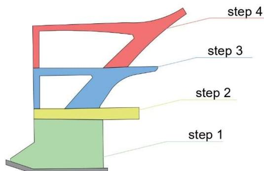
Figure 24 inclined pillars construction steps scheme
