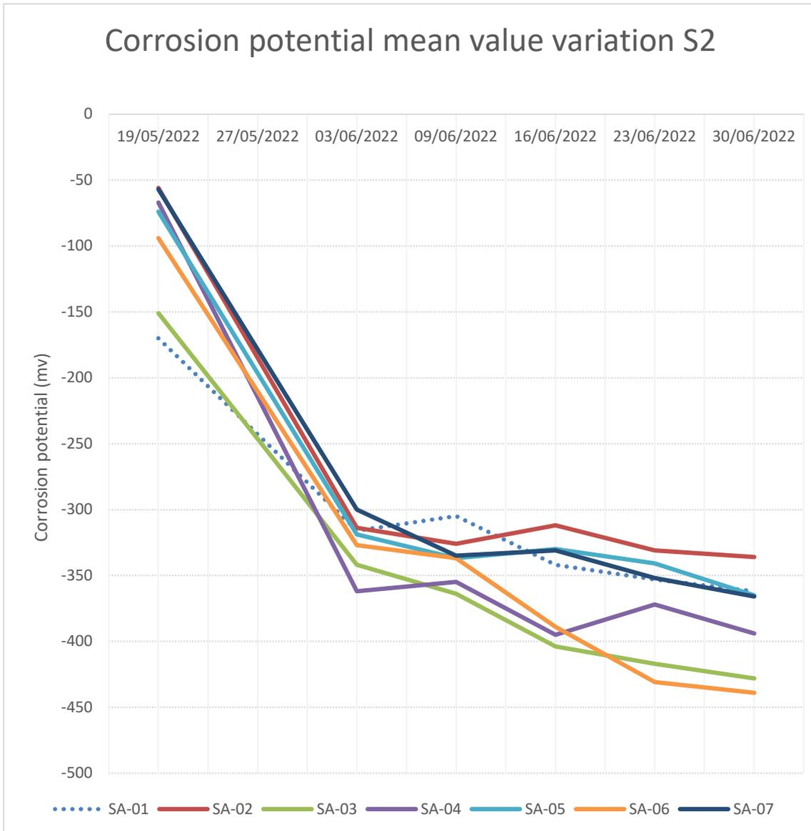
Figure 68 S2 mean corrosion potential variation
