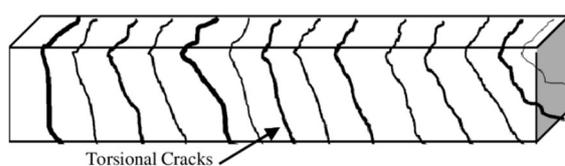
*Figure 6 torsional cracks shape [9]*
