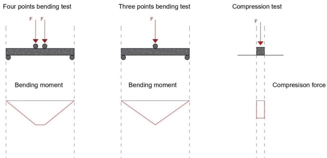
*Figure 57 different tests configuration*
