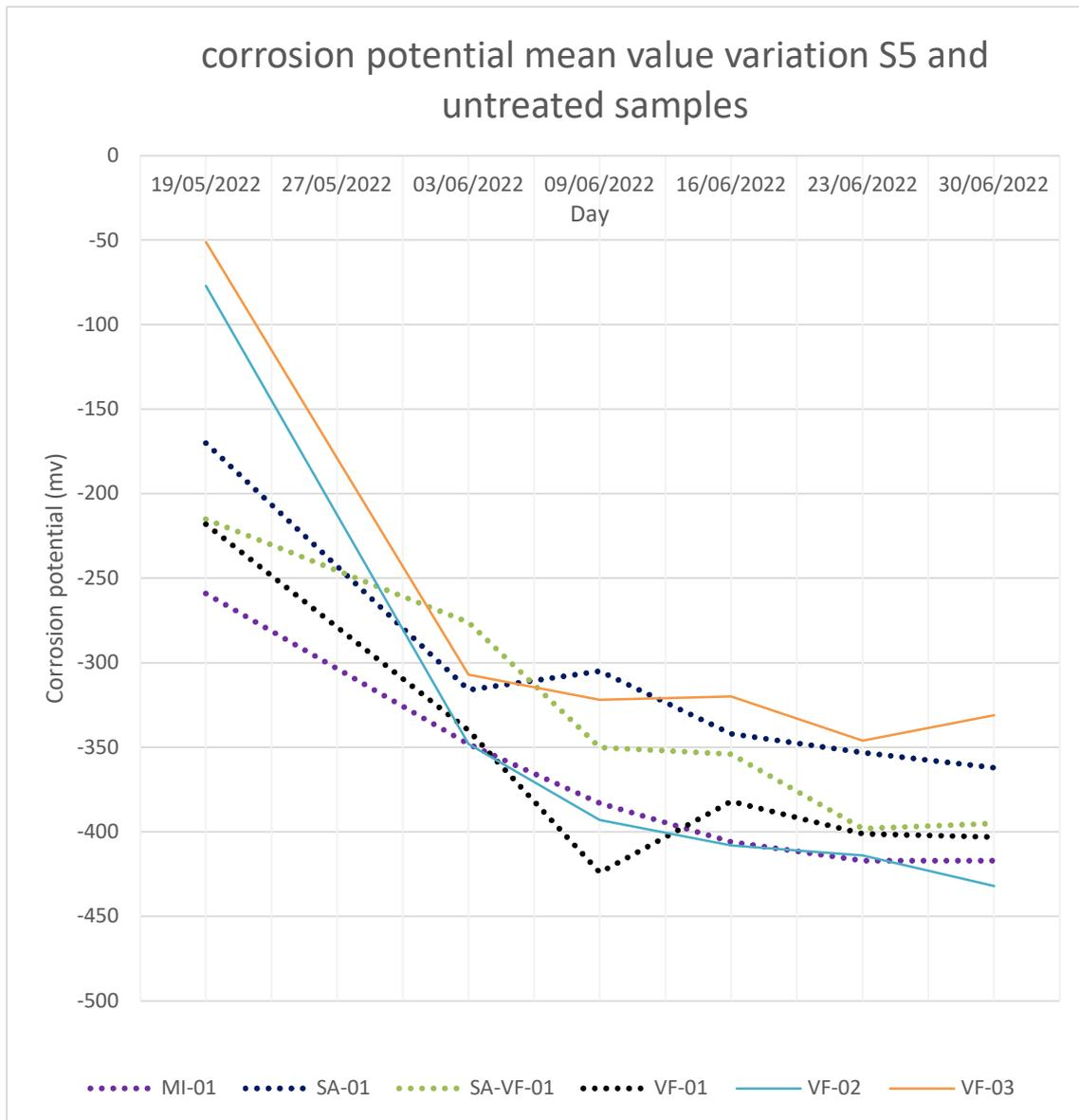
Figure 71 S5 and untreated samples corrosion potential mean values variation
