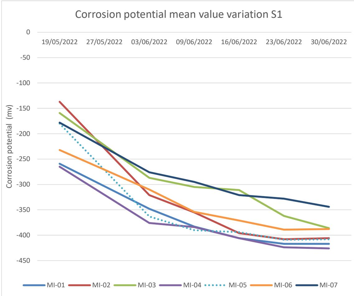
Figure 80 S1-M1 corrosion potential mean values
