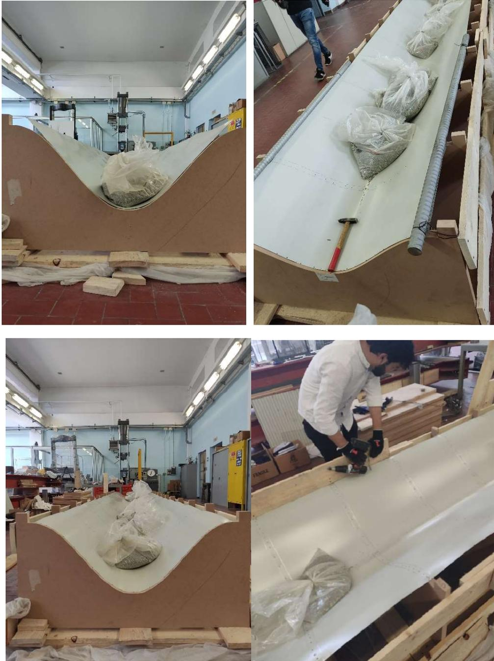
*Figure 60 from up on the left: Fixing in the middle point of the middle of the plate, side fixing of the plate by using steel bars, final shape, side wood boards positioning*
