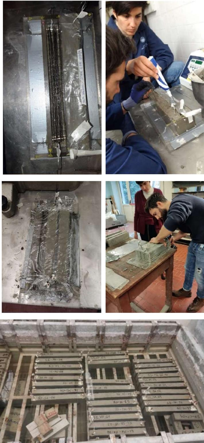
*Figure 50 Ferrocement samples casting steps: from up left to down right: (i) steel net package inserting, (ii) concrete final compacting procedure, (iii) concrete samples covering, (iv) de-assembling formwork, (v) underwater curing*
