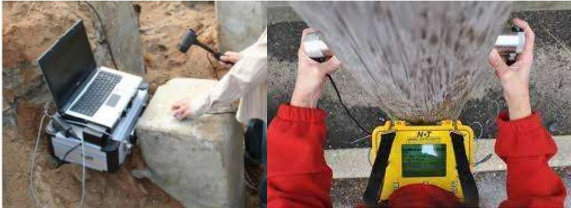
Figure 15 impulsive response test [15] (left), ultrasonic test [26] (right)
