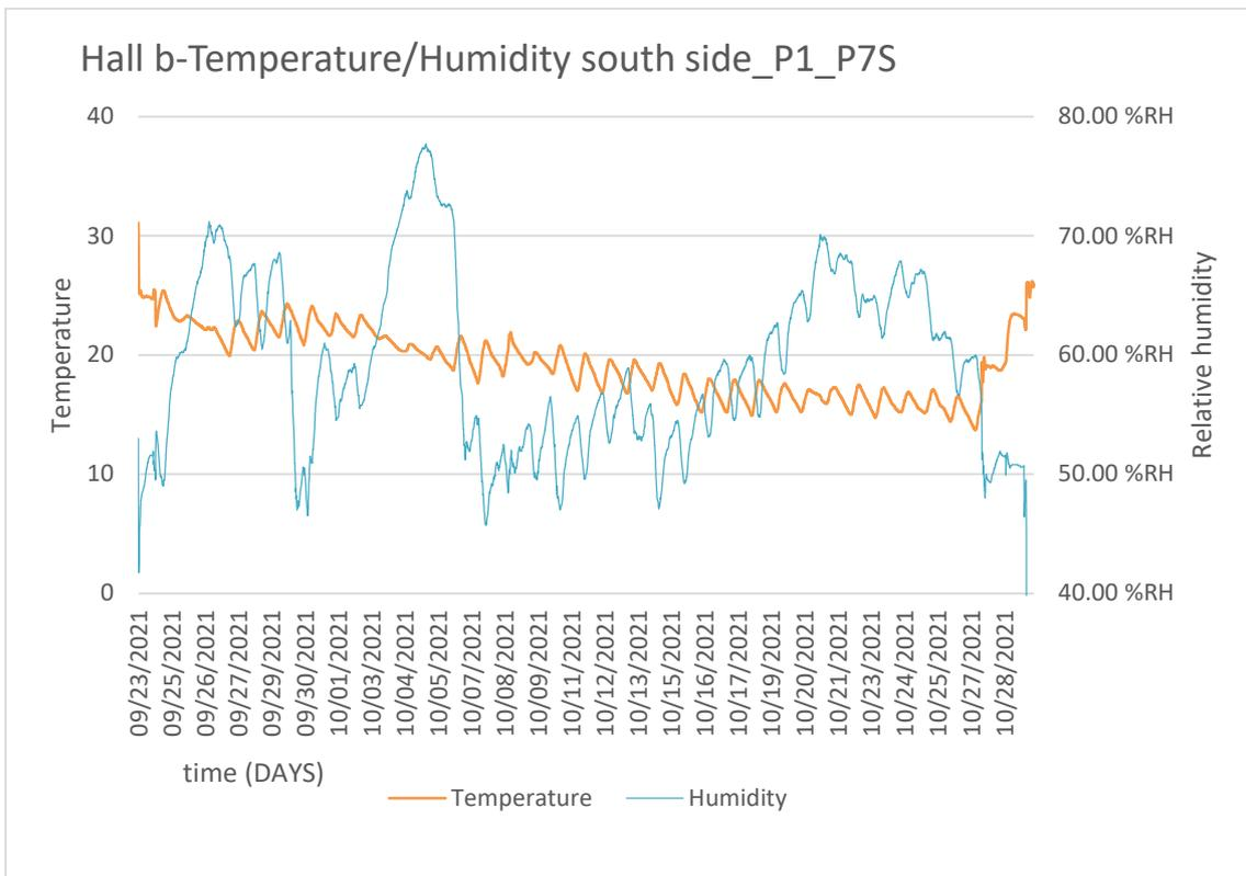
Figure 36 Hall B P1\_P7S Temperature and humidity sensor output
