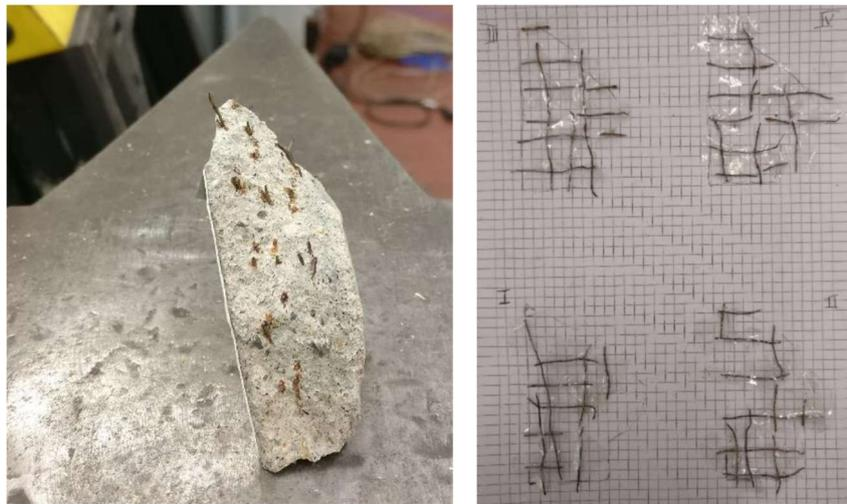
Figure 40 on the left: ferrocement sample, on the right: ferrocement wire meshes extracted from the sample [39]
