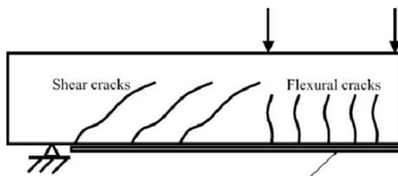
*Figure 4 shear and flexural cracks shape [9]*
