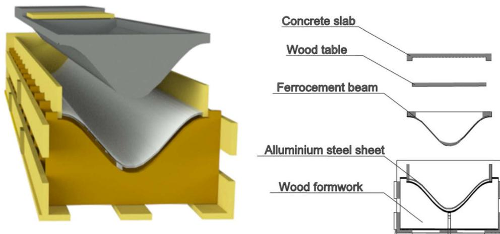
*Figure 58 up: ferrocement beam realization, low: ferrocement formwork model and section*
