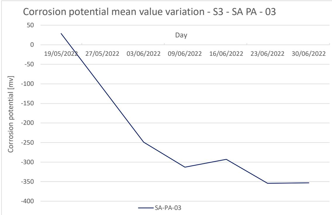
Figure 89 S3-PA SA-03-corrosion potential mean value variation
