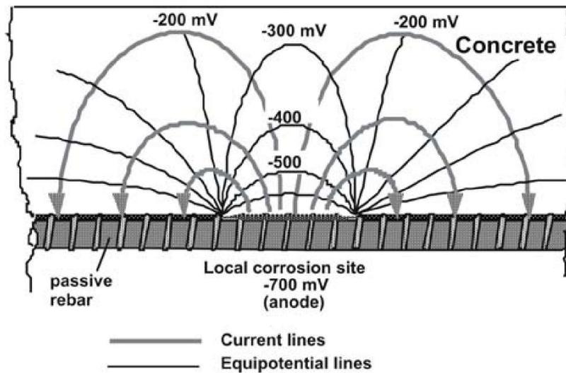
Figure 12 corrosion potential level map on steel and concrete [20]
