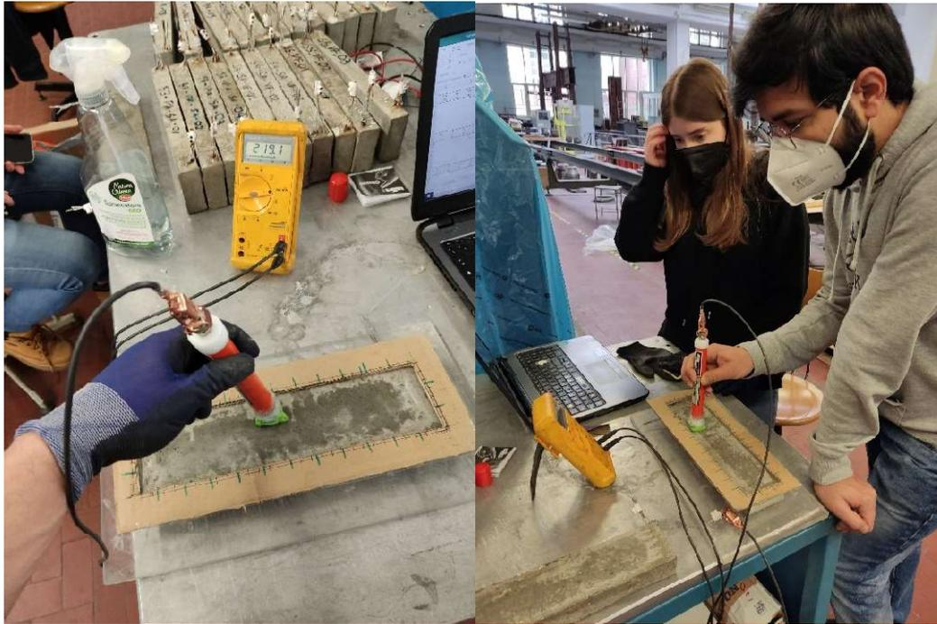
Figure 53 Corrosion Potential Measurement
