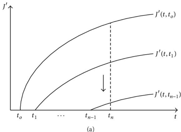
Figure 9 Creep deformation / time graph, curves for different time of application of the first load on the specimen [11]
