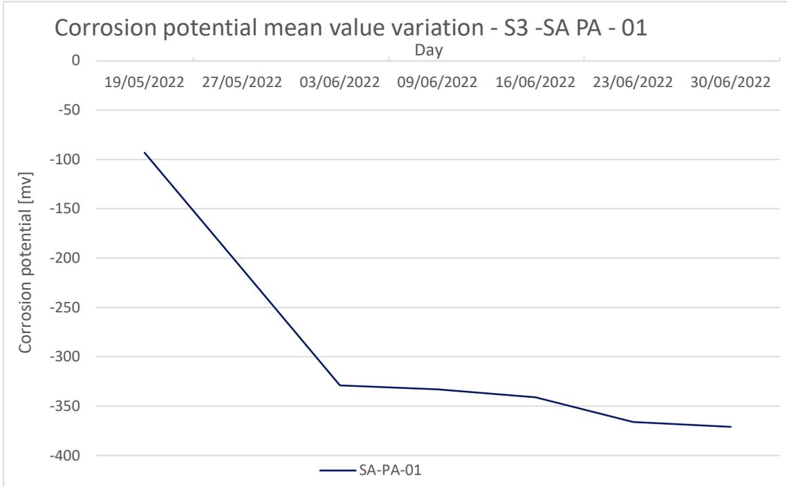
Figure 88 S3-PA SA-01- corrosion potential mean value variation
