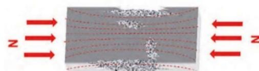
*Figure 5 compression crack lines [4]*
