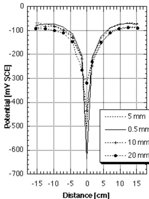
Figure 13 cover depth influence on the half-cell corrosion potential [21]
