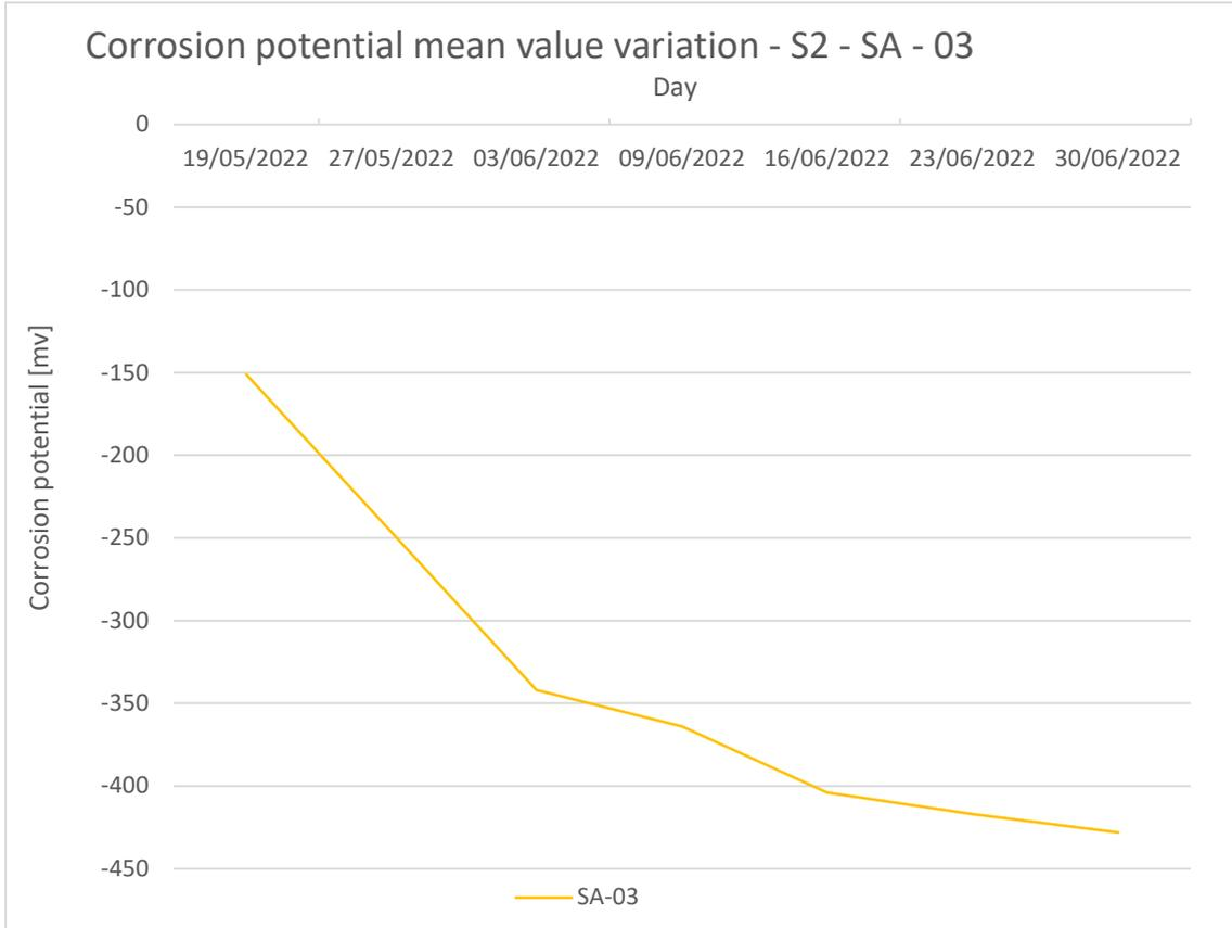
Figure 82 Table 81 S2-SA-03 corrosion potential mean value variation
