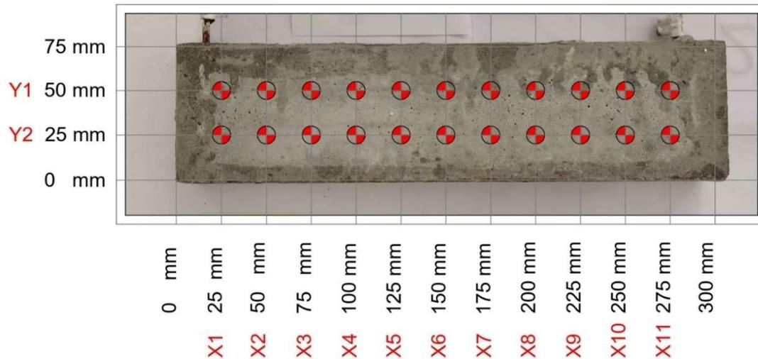
Figure 64 corrosion potential measurements scheme
