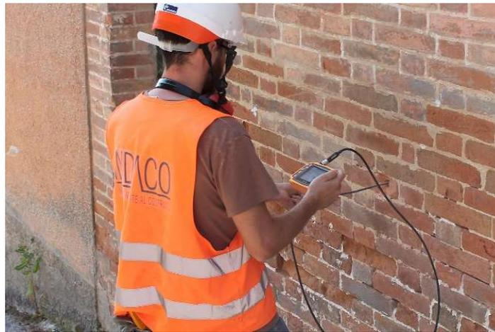
*Figure 10 endoscopy test [17]*
