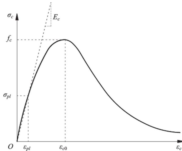
Figure 19 stress-strain compression behaviour in concrete [30]
