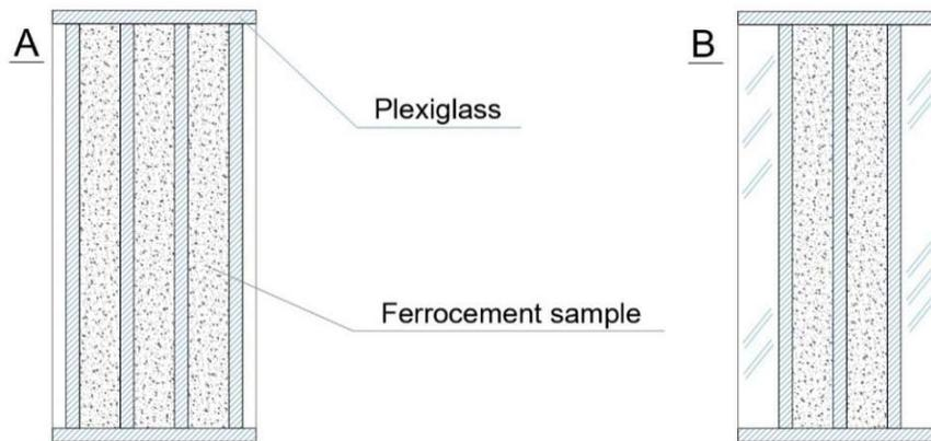
Figure 46 Plexiglass formworks type A and B
