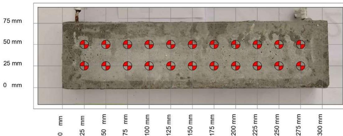
Figure 54 corrosion potential sampling scheme
