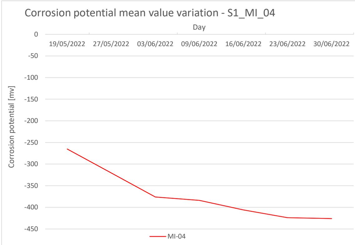
Figure 76 S1-M1-04 corrosion potential mean values
