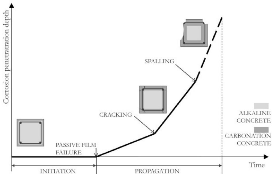
*Figure 3 Corrosion development in reinforced concrete*
