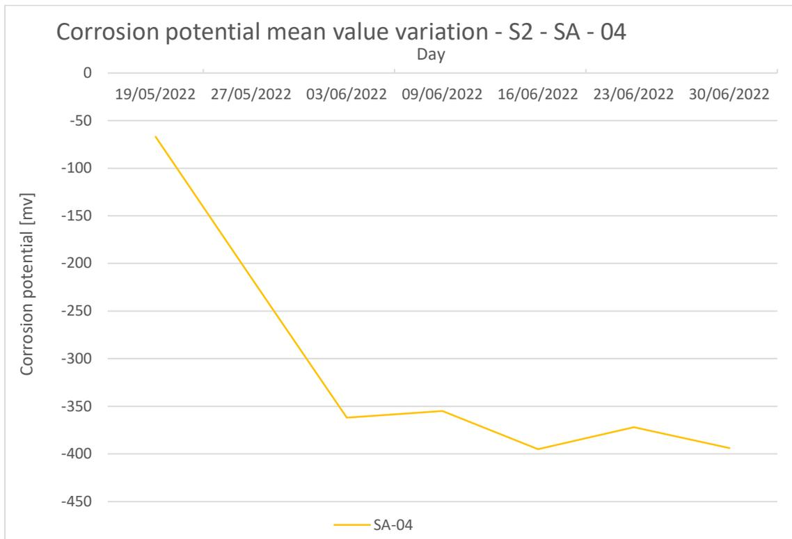
Figure 83 S2-SA-04- corrosion potential mean value variation
