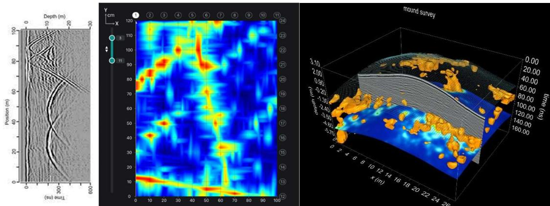
Figure 14 Different georadar scan output, from the left: 1D scan [24], 2D scan and 3D scan [25]
