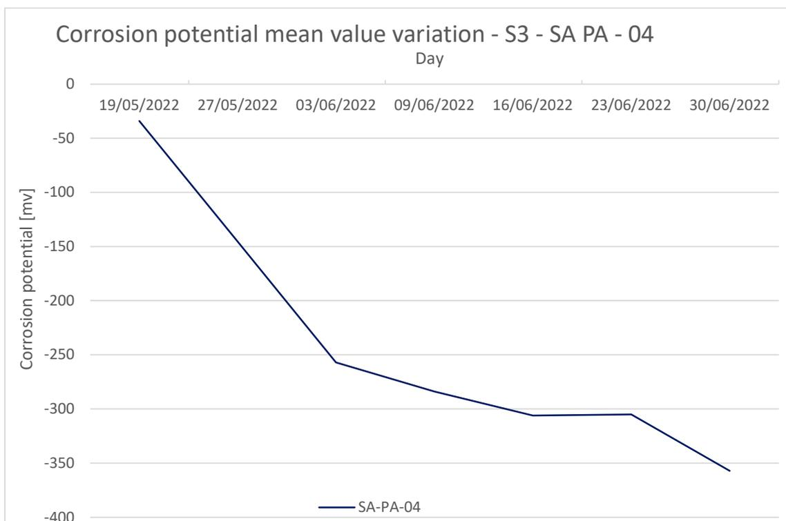
Figure 90 S3-PA SA-04-corrosion potential mean value variation
