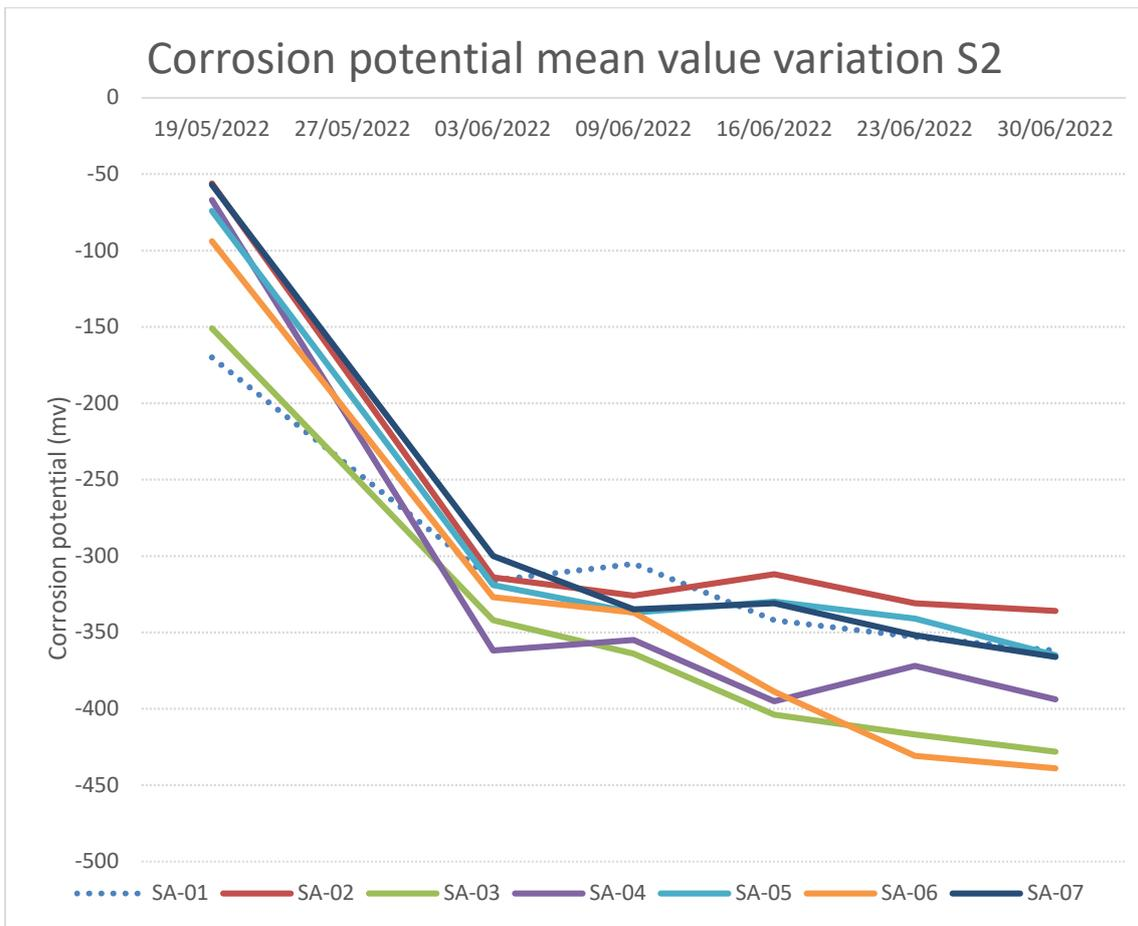
Figure 87 S2-SA- corrosion potential mean value variation
