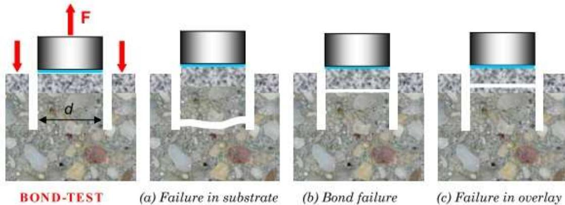
Figure 18 Pull-off test scheme and possible failure mechanisms [29]
