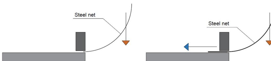
*Figure 43 Steel sheet bending scheme*
