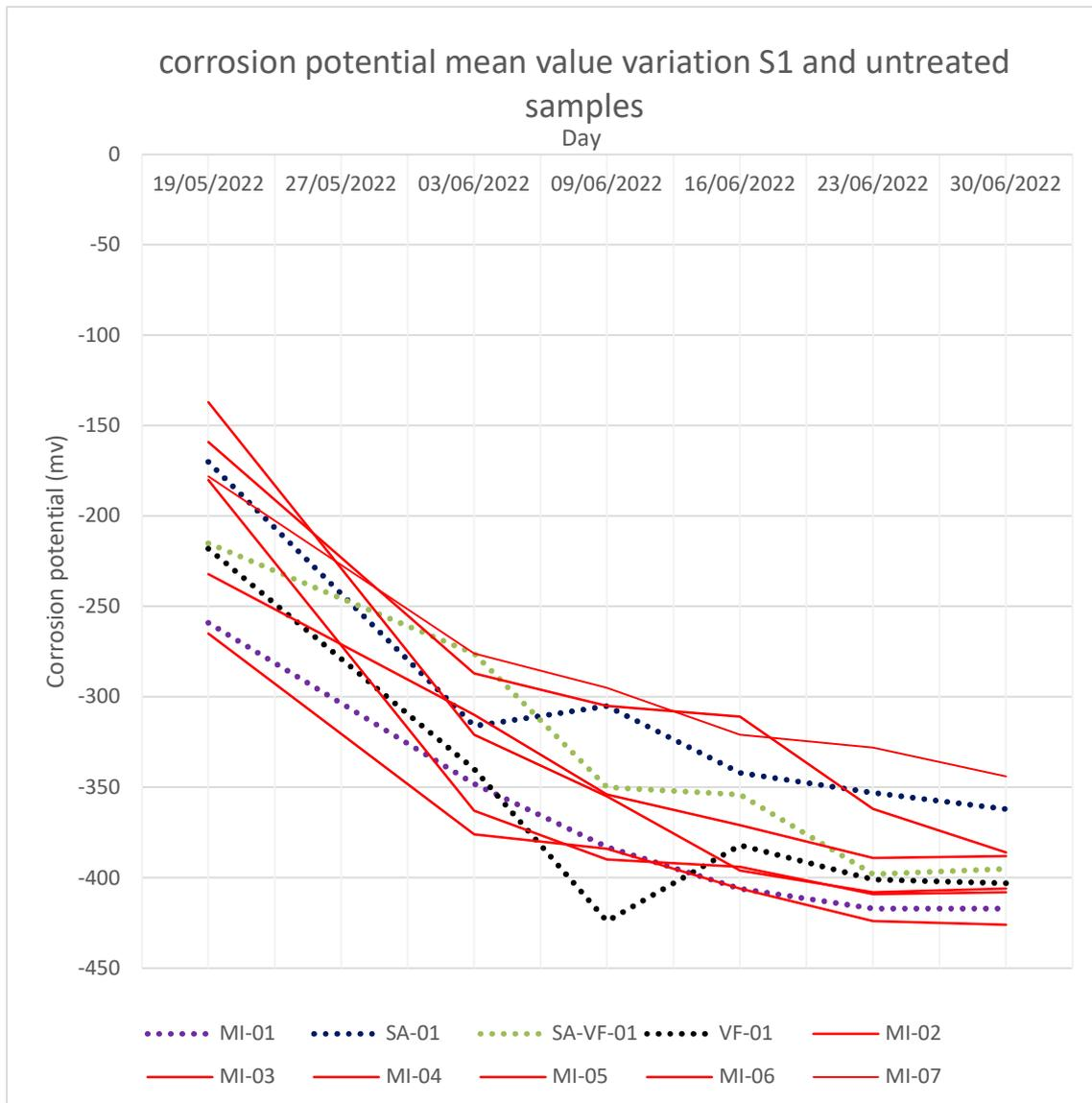
Figure 65 S1 and not treated samples mean corrosion potential values variation
