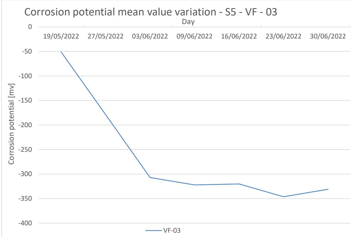
Figure 96 S5-VF-03-corrosion potential mean value variation
