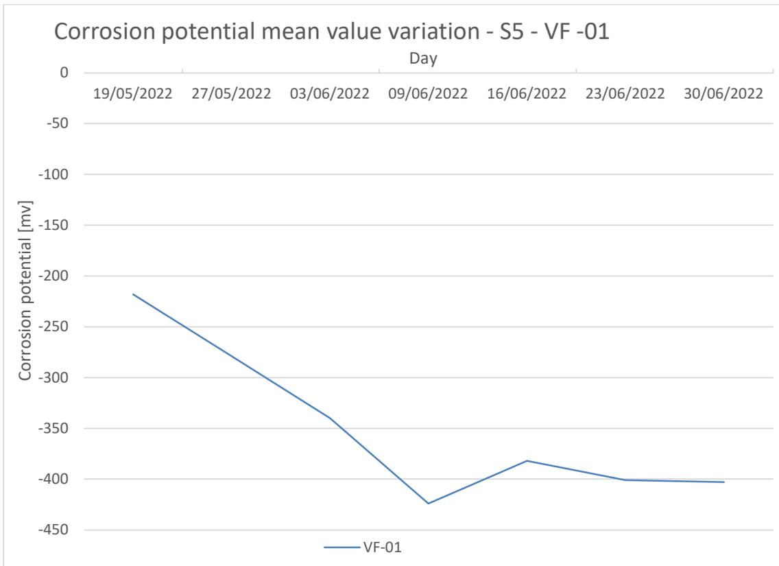
Figure 95 S5-VF-01--corrosion potential mean value variation
