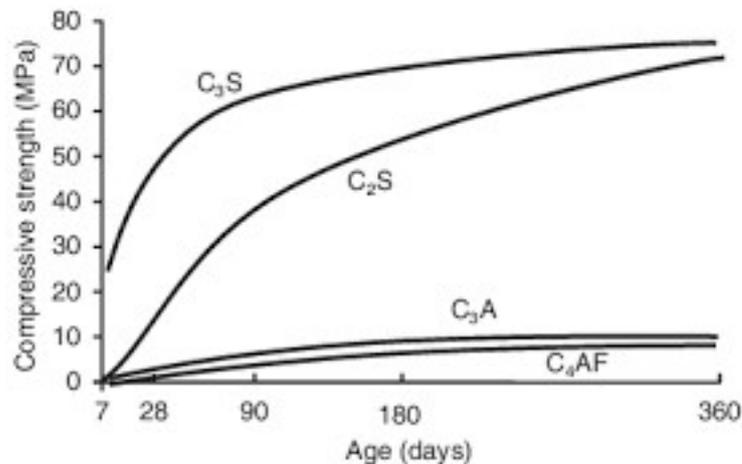
Figure 1 elements compressive strength development vs time [2]
