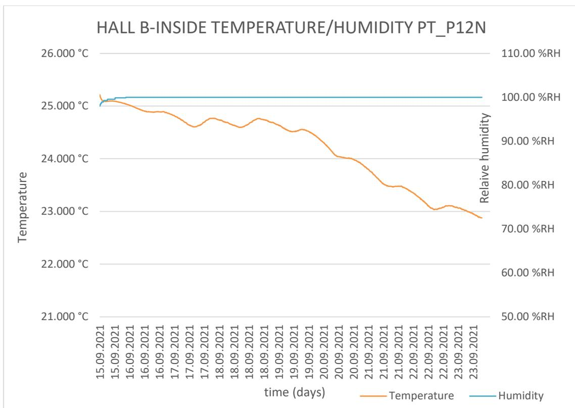
Figure 35 PT\_P12N Hall B temperature/humidity sensor output
