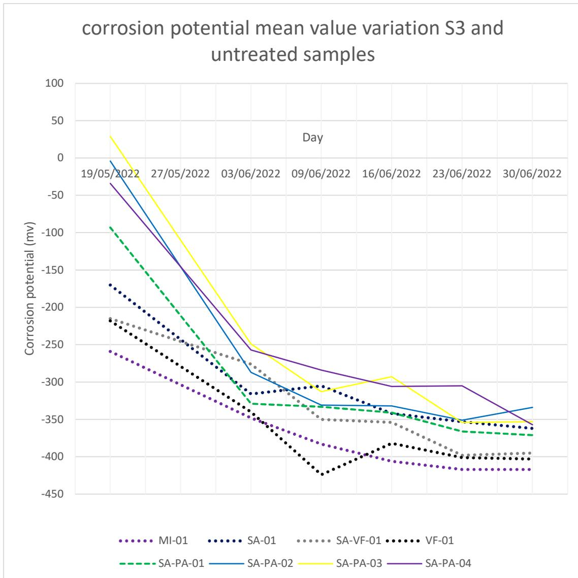
Figure 69 S3 and untreated samples corrosion potential mean values variation
