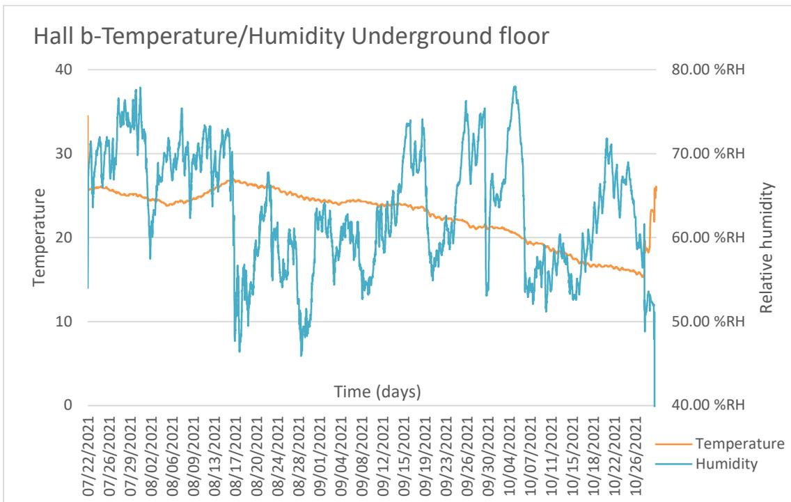
Figure 37 Hall B underground floor pillar temperature/humidity sensor output
