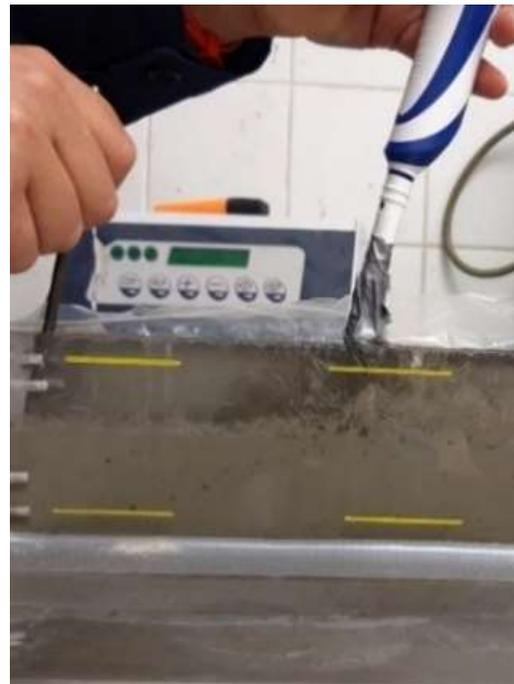
*Figure 49 Ferrocement samples casting procedure, from up left to down right: (i) oil-based release agent application on formwork, (ii) concrete mix weighting (iii) water weighting (iv) compacting concrete*
