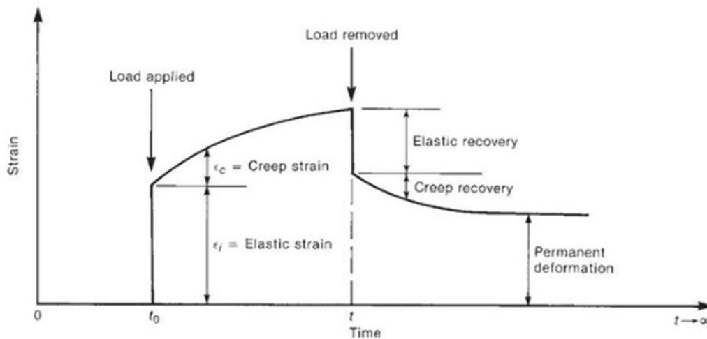
Figure 8 creep deformation time / strain graph [10]
