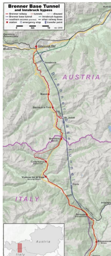
Figure 1 – map of the Brenner Base Tunnel (blue, under construction) and Innsbruck bypass (green), side by side with the Brenner railway (OpenStreetMap, Eigenes Werk)
