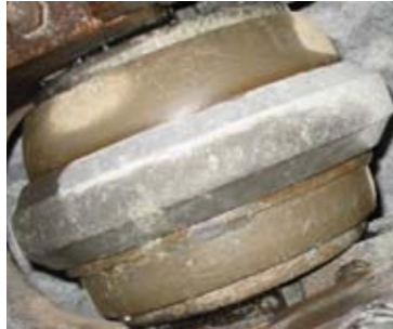
Figure 57 - Cutter normal wear (Herrenknecht, S-1054 TBM GL Brenner Basis Tunnel Lot 2-3 Mauls/Mules, 2017)
