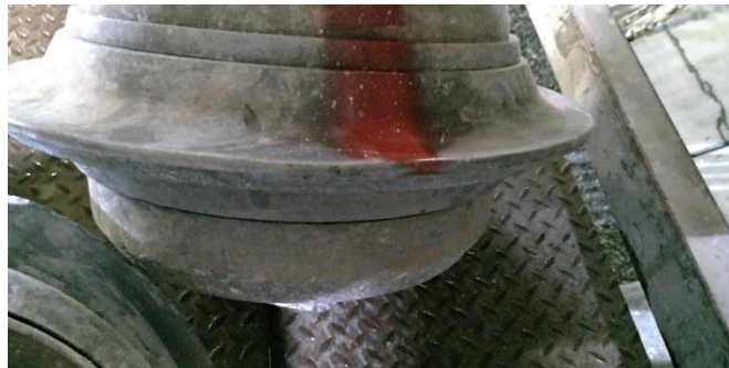
Figure 62 - Defective roller casing
