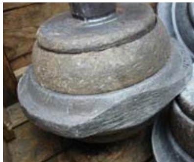
Figure 58 - Cutter clogging bearing (Herrenknecht, S-1054 TBM GL Brenner Basis Tunnel Lot 2-3 Mauls/Mules, 2017)
