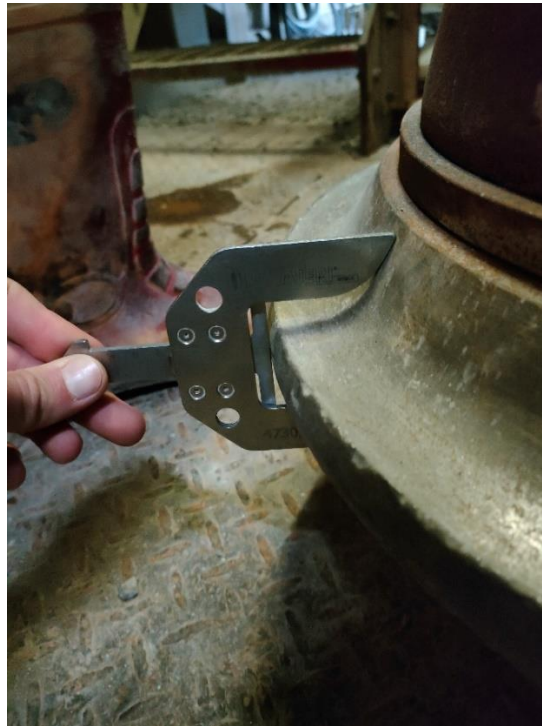
Figure 56 - Wear gauge template for cutter ring wear measurement
