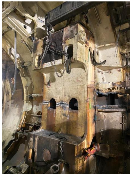
Figure 39 - gripper shoes dismantling
