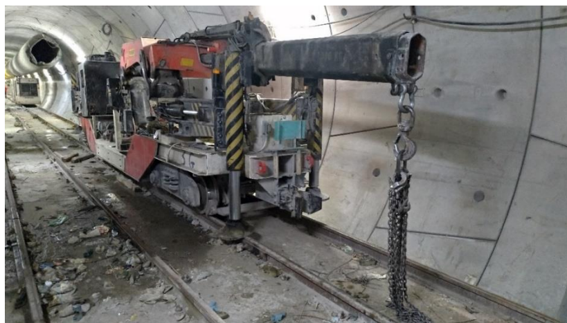
Figure 35 - train crane used during the disassembly
