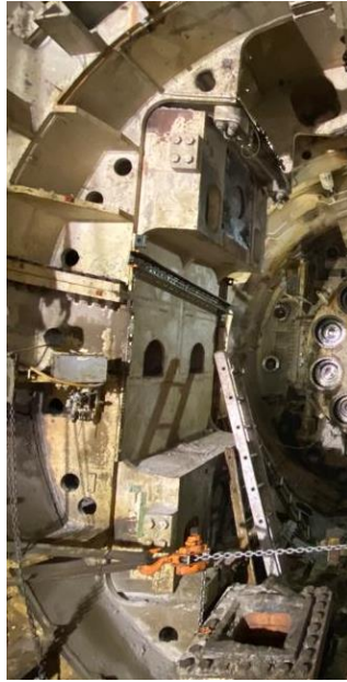
Figure 38 - gripper shoe safe to the TBM shield by means of a steel beam
