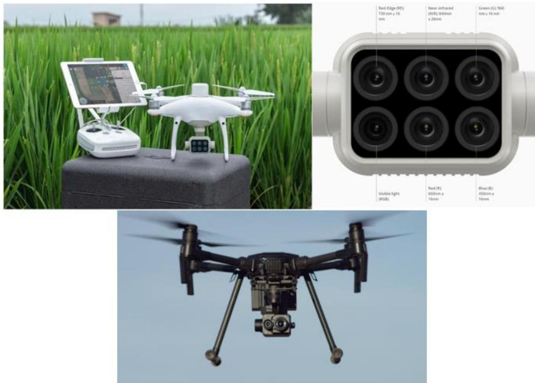
Figure 1. Up left: DJI phantom4 camera, up right: 6 spectral bands of phantom4 drone, bottom: Thermal camera XT2
