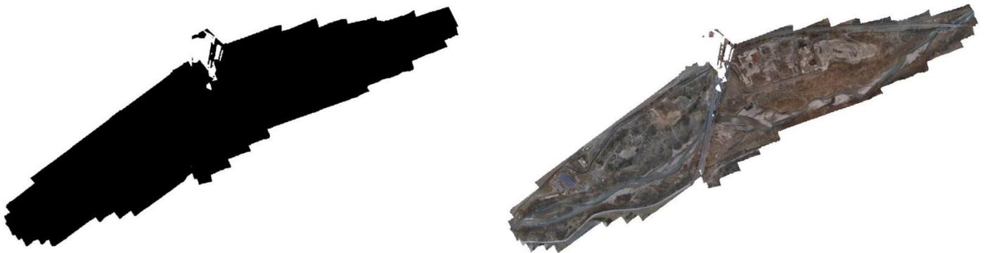
Figure 22. Orthomosaic- left: NIR Band, right: RGB band
