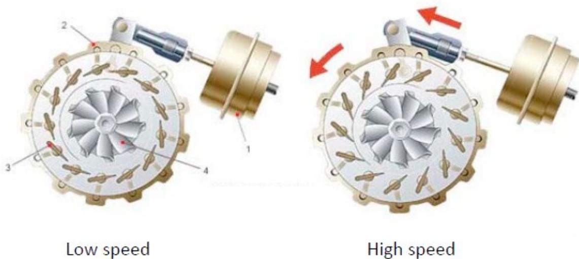
Figure 2.10 VGT configurations at two different speeds at full load [8]
