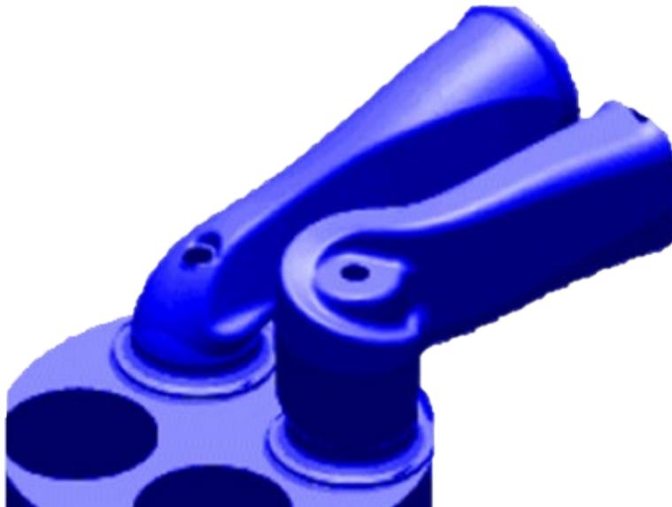
Figure 2.19 An example of intake ports geometry to increase swirl motion: direct and helical ports combo [8]
