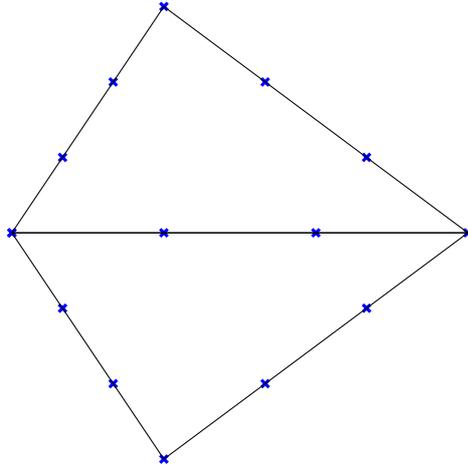
Figure 2.7: The figure shows the two elements and their degrees of freedom (represented with blue crosses).
