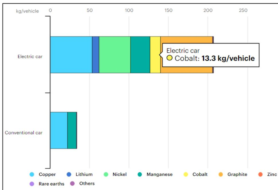
Fig. 31. Minerals used in electric cars compared to conventional cars [37]
