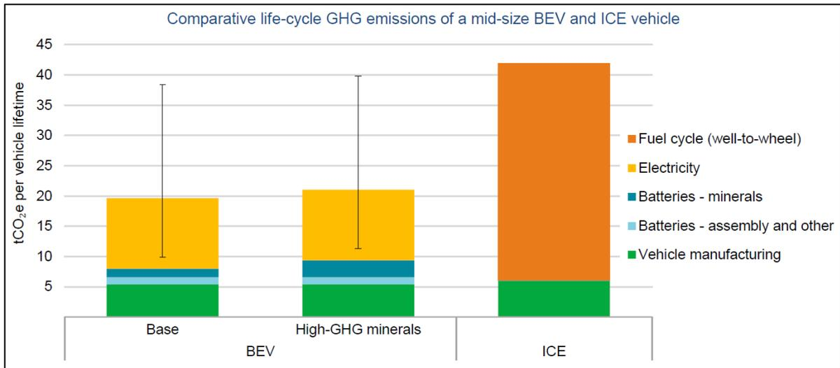
Fig. 60. Comparative life-cycle GHG emissions of a mid-size BEV and ICE vehicle [37]
