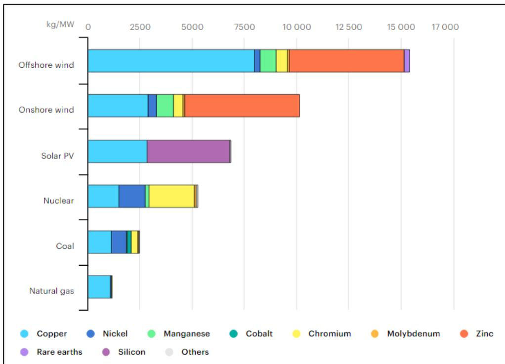
Fig. 30. Minerals in renewable technologies compared to other power generation sources [37]
