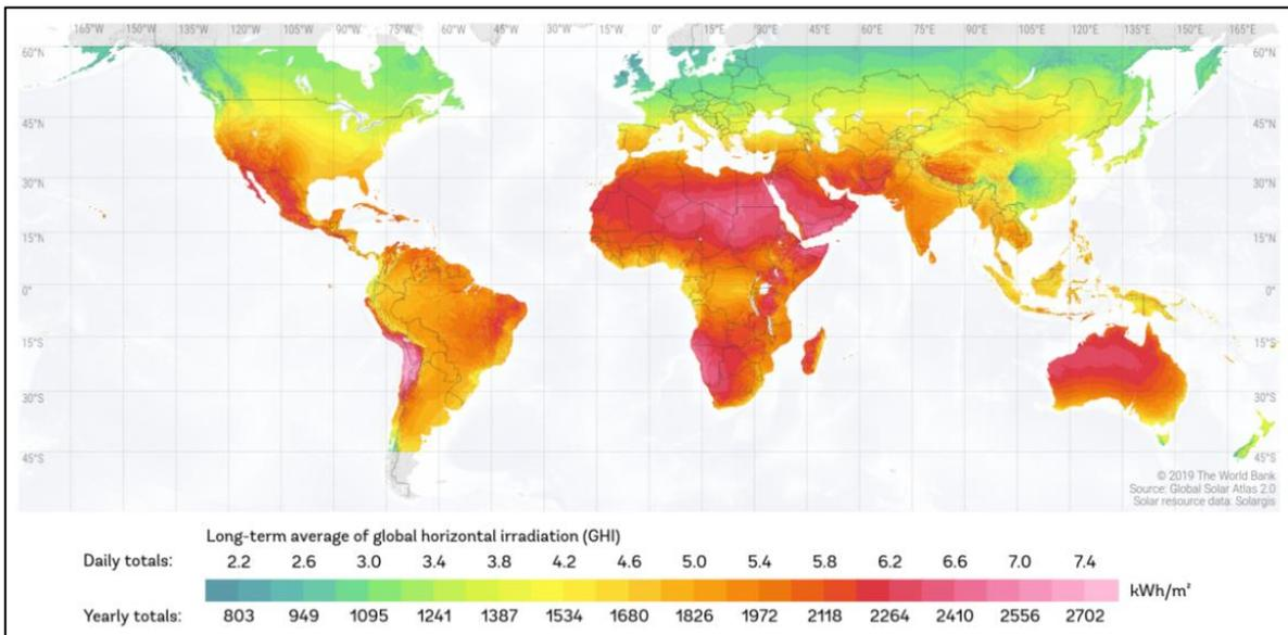
Fig. 21. Solar resource map: global solar irradiation [32]
