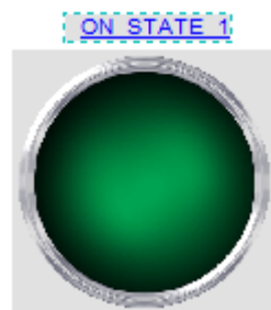
Figure 99: Indication of the assignment (the blue alias) in AS software
