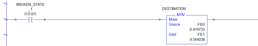
Figure 130: Showing the value of the pressure when the system is in the broken state
