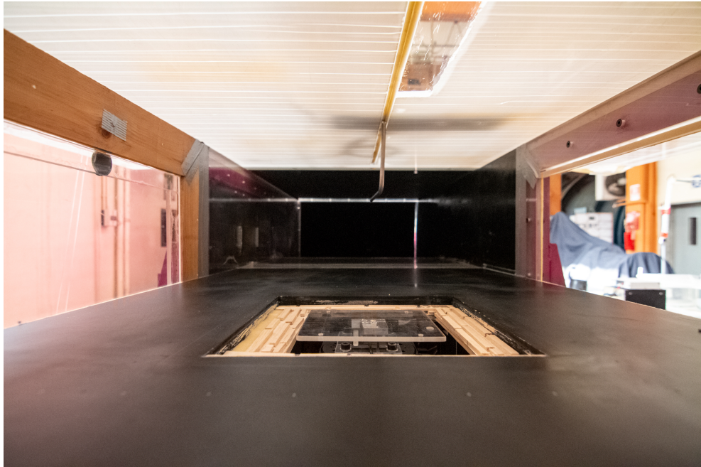
Fig. 4.5: Inside view of the testing chamber. Flow is moving towards the viewer. It's noticeable the labyrinth in the hole for the plaques.
