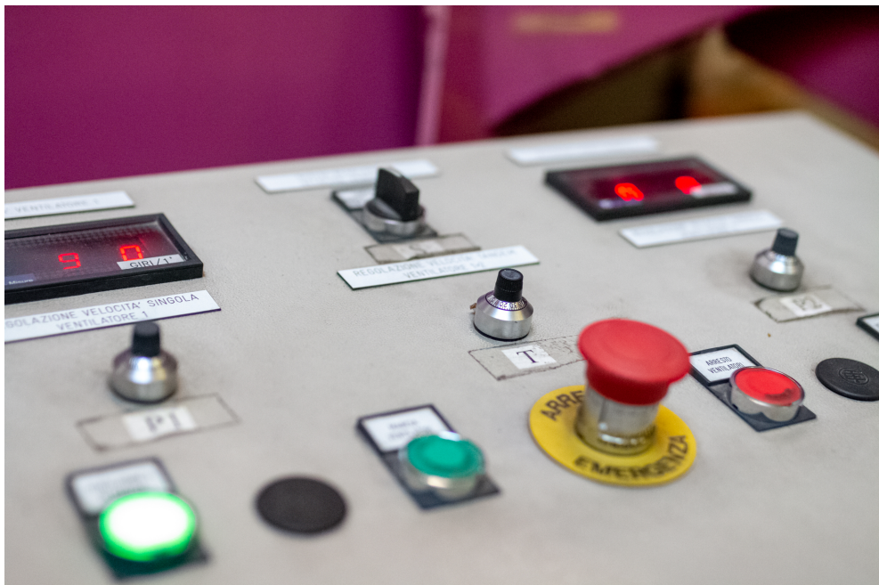
Fig. 4.9: The wind tunnel control panel, with the various controls for each motor and the two displays.
