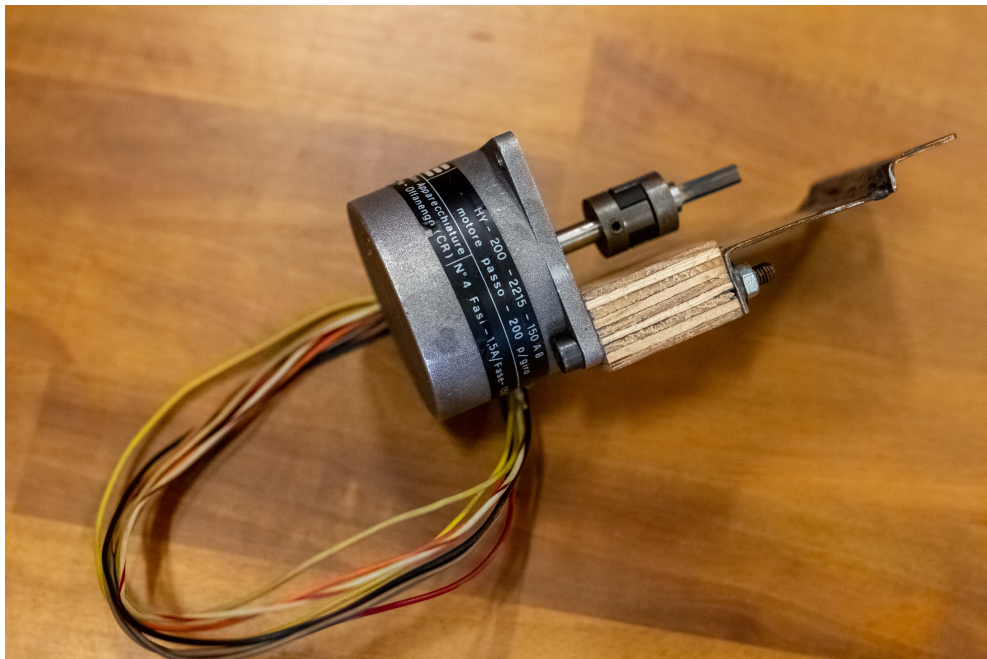
Fig. 4.21: Stepping motor MAE HY-200-2215-A-8, used to change the y position of the plaque.
