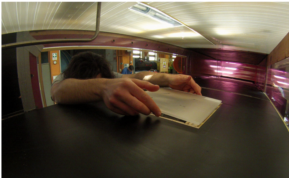
Fig. 4.33: Manual positioning of the test plaque onto the acrylic interface, making sure to intercept the metal gaskets.
