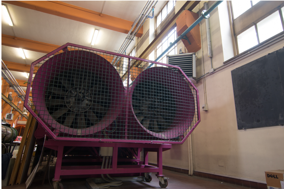
Fig. 4.2: Inlet and rotors of the wind tunnel.
