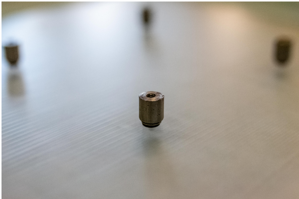
Fig. 4.13: Close up view of the four threaded sockets, used to attach the plaque to the force sensor.
