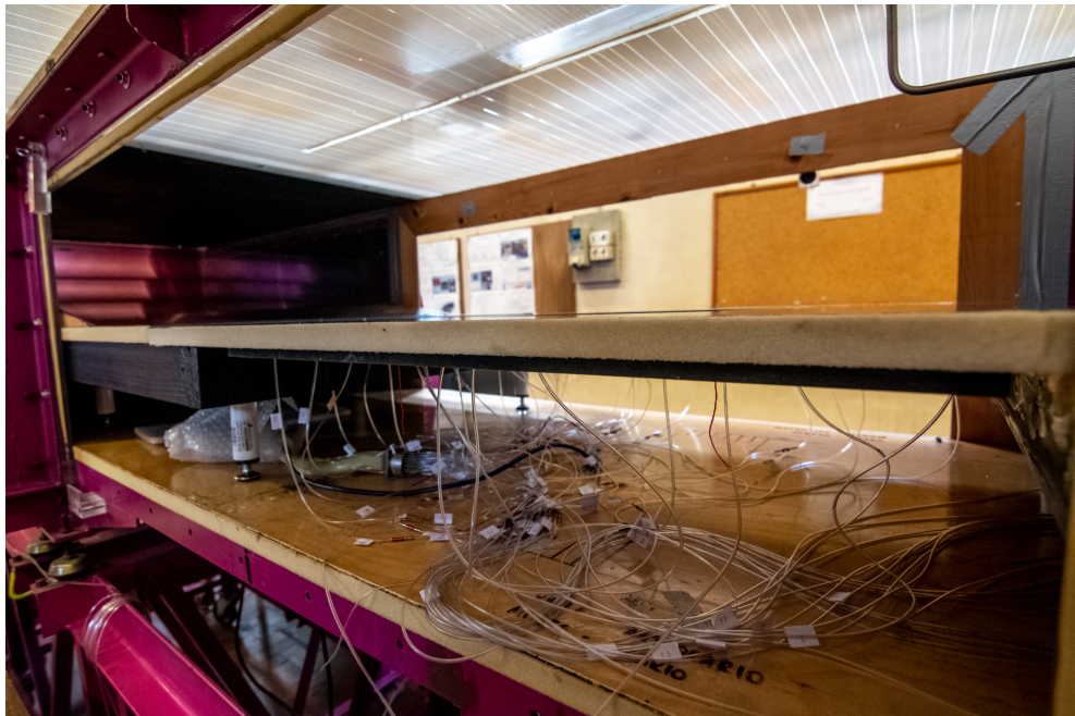
Fig. 4.4: Closer view of the testing chamber with the medium density fiberboard in the middle of the frame. From it, the various tubes for measuring the pressure gradients hang.
