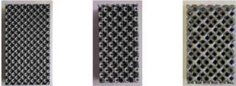
Figure 33 Provini ROM in AlSi10Mg da 3mm, 5mm e 7mm
