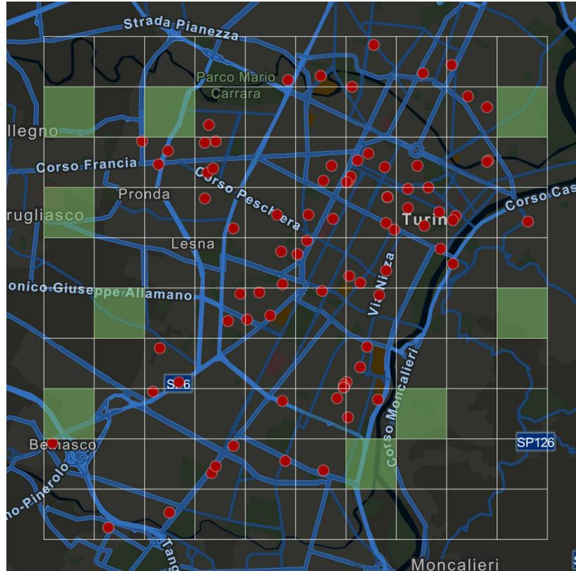
Figure 6: A preliminary selection for possible locations of new EV charging infrastructure in Turin on a 1km<sup>2</sup> grid based on the baseline tuning parameters.
