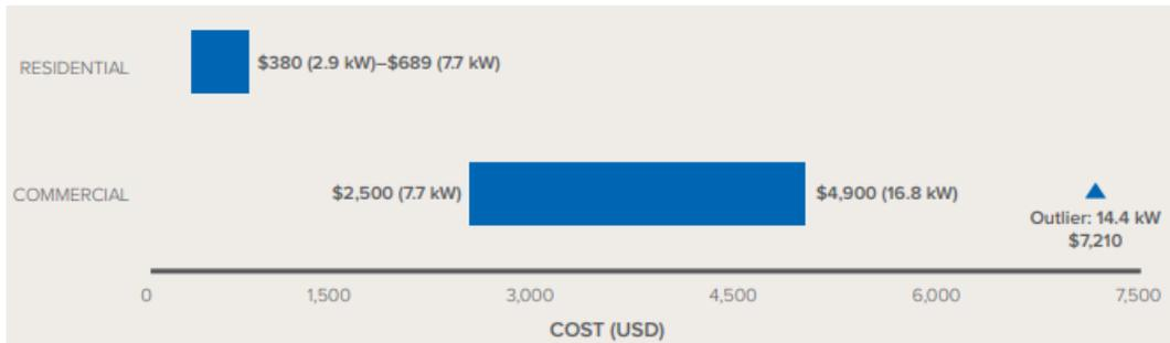
Figure 2: An overview of the range of costs associated with installing a traditional AC charger (Nelder and Rogers, 2019).
