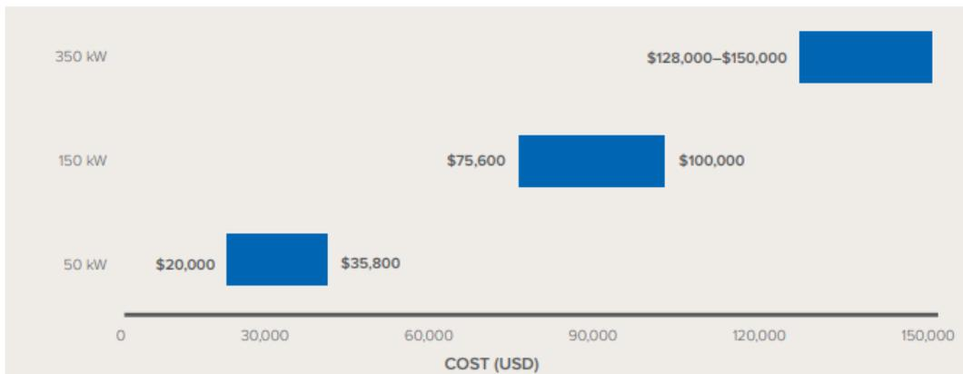
Figure 3: An overview of the range of costs associated with installing a direct current fast charger (Nelder and Rogers, 2019).
