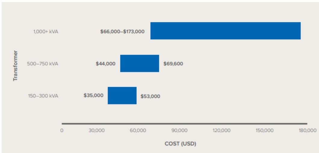
Figure 4: An overview of the range of costs associated with upgrades to distribution transformers, should these be required for new EV charging infrastructure (Nelder and Rogers, 2019).
