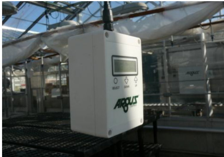
Figure 6.10: Aspirated box with digital output screen in greenhouse.
