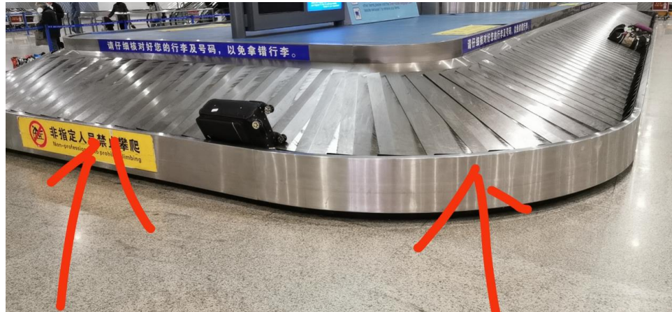
Figure 16: Stainless steel from airport baggage conveyor belt, radar can't correctly scan surface mirror-reflected objects.
