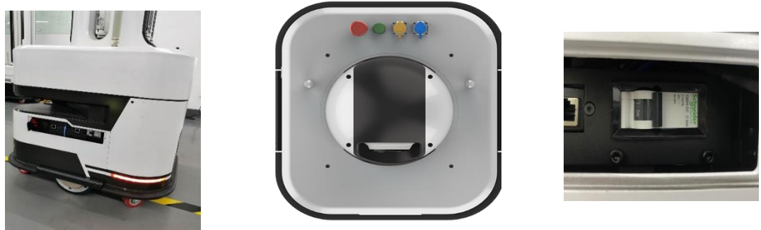
Figure 7: Robot EM state, buttons and ports, air switch.
