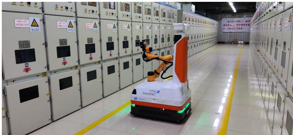
Figure 15: Corridor longer than lidar scanning range, and AGV two sides of the travel without obvious feature reference.
